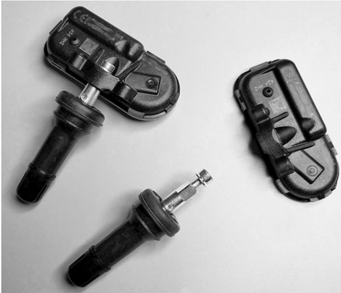
Figure 12-3: Two TPMS sensors
