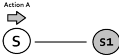
Figure 3-2. Deterministic environment; an agent is in state S and can only move to state or percept S1 after executing an action A. Every state is linked to just one state; i.e., there's a single possible outcome for every action executed by the agent.
