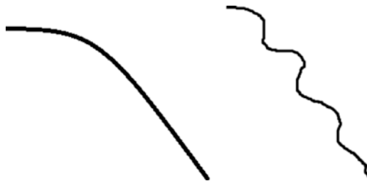
Figure 11-9. To the left the direct path that GDS would follow over the error surface to get to a minimum; to the right the “unbalanced” path followed by SGD
