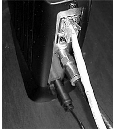
Figure 6.10 The cable modem is simple to connect and set up. The connection to the PC or laptop is done typically by utilizing LAN or USB cable, and the connection up to the server of the service provider happens via the television cables.
