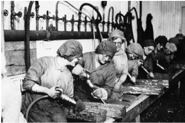
Women workers in ordnance shops, Midvale Steel and Ordnance Co., Nictown, Pa. Hand chipping with pneumatic hammers. 1918. National Archives and Records Administration
