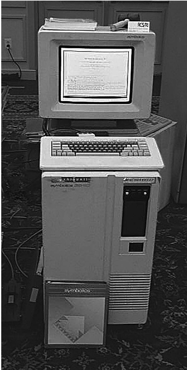
A Symbolics Lisp Machine: An Early Platform for Expert Systems. Note the unusual "space cadet keyboard". (wikipedia). Michael L. Umbricht and Carl R. Friend (Retro-Computing Society of RI)
