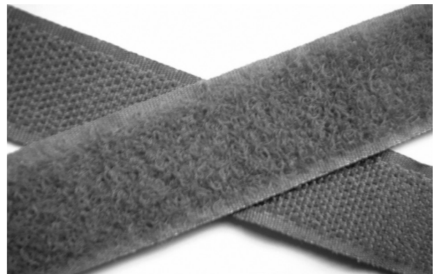
Velcro tape mimics biological examples of multiple hooked structures such as burs. By Ryj (Own work)
