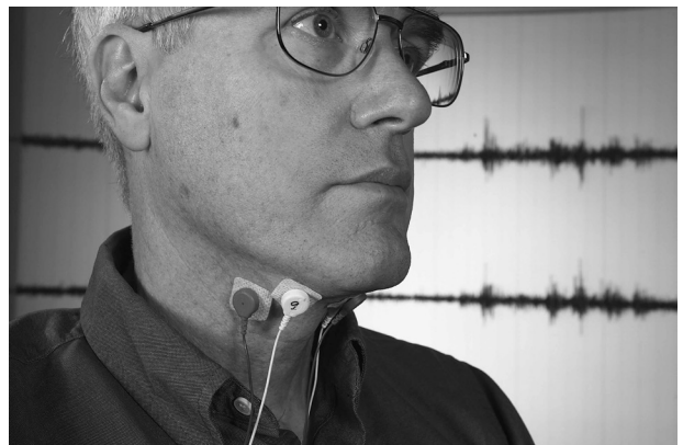
Electrodes used in subvocal speech recognition research. By Dominic Hart, NASA
