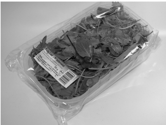
Packaging blister made by bioplastics (Celluloseacetat). By Christian Gahle, nova-Institut GmbH (Work by Christian Gahle, nova-Institut GmbH)
