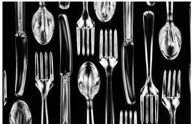
Knives, forks, and spoons made from a biodegradable starch-polyester material. By Scott Bauer
