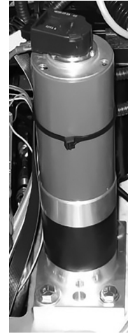
An industrial servomotor. The grey/green cylinder is the brush-type DC motor, the black section at the bottom contains the planetary reduction gear, and the black object on top of the motor is the optical rotary encoder for position feedback. By John Nagle (Own work)
