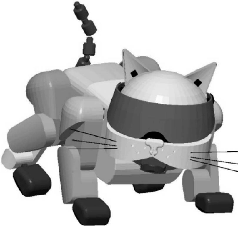
Fig. 7: Mechanical design of robot kitten “Robokitty”
