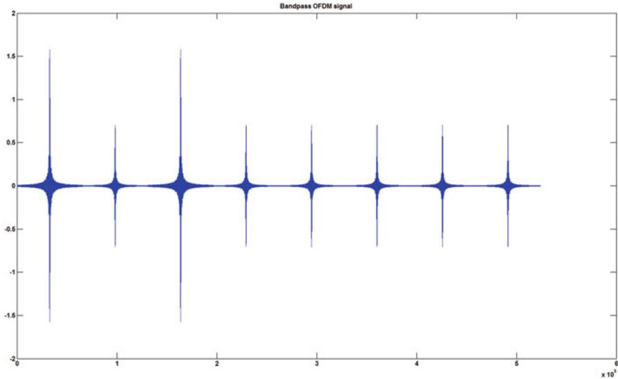
**Fig. 3.28** Bandpass OFDM signal using sinc pulse to represent the in-phase and the quadrature components
