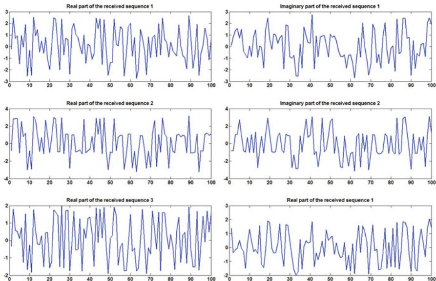
Fig. 1.20 Received base band MIMO signal with additive Gaussian noise
