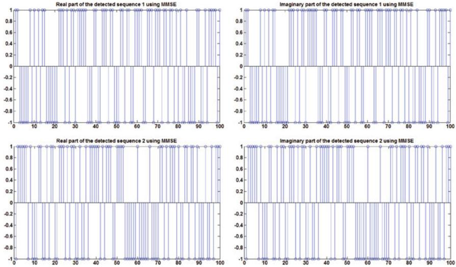
**Fig. 1.26** Detected data sequence in the MIMO set-up using Linear MMSE (computed using  $p_d$ ) (which is identical as that of Fig. 1.19, i.e. with zero error)
