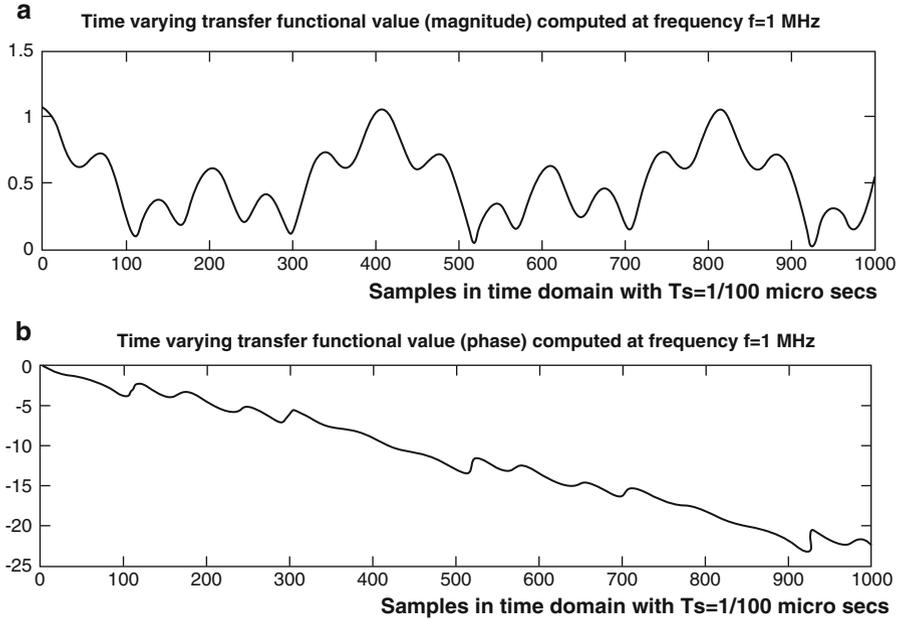
**Fig. 1.7** Illustration of the fast fading channel characteristics
