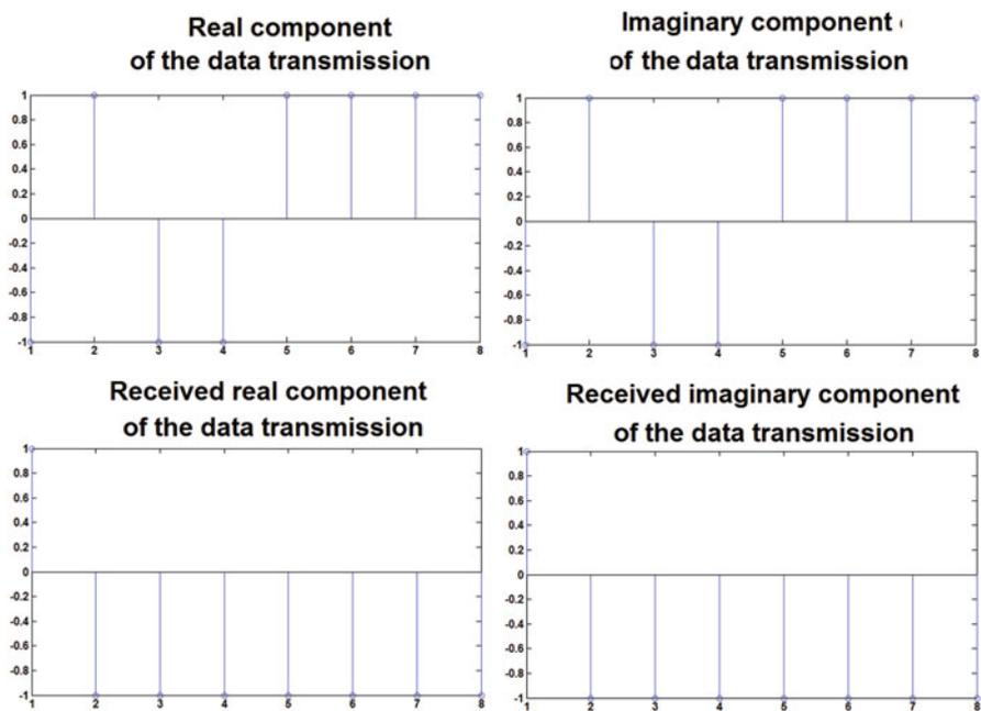
Fig. 3.30 Illustration of the detection of I- and Q-component from the noisy received OFDM signal
