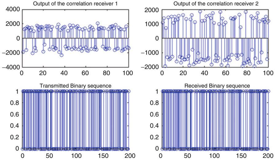
Fig. 3.22 Illustration of the correlation receiver of the QPSK signal
