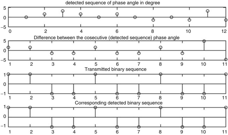
**Fig. 3.18** Steps involved in detecting binary sequence from MSK signal
