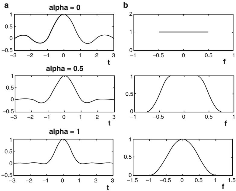
**Fig. 3.2** (a) Truncated modified pulse with  $T_b = 1$  in time domain. (b) Modified pulse in frequency domain with  $W = 1/2$ . It is noted that bandwidth increases from  $W$  to  $2W$  as  $\alpha$  goes from 0 to 1
