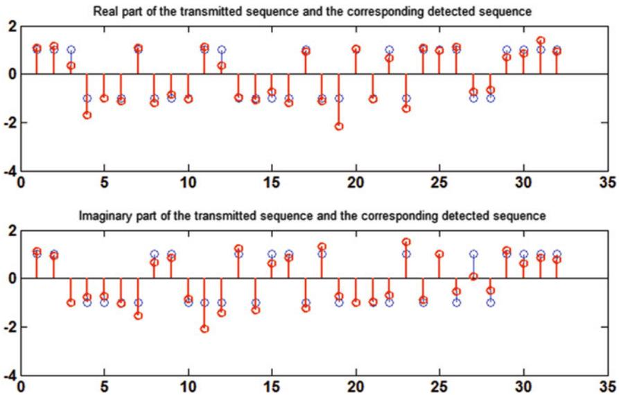
Fig. 3.32 Illustration of discrete data transmission using OFDM
