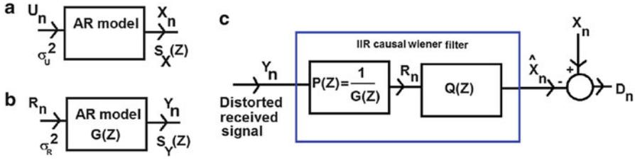
**Fig. 2.14** Illustration of causal IIR Wiener filter-based estimation
