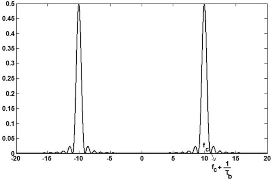
Fig. 3.8 Spectral density of the PSK signal with  $E_b = 1$  unit,  $T_b = 1$  unit and  $f_c = 10$  units
