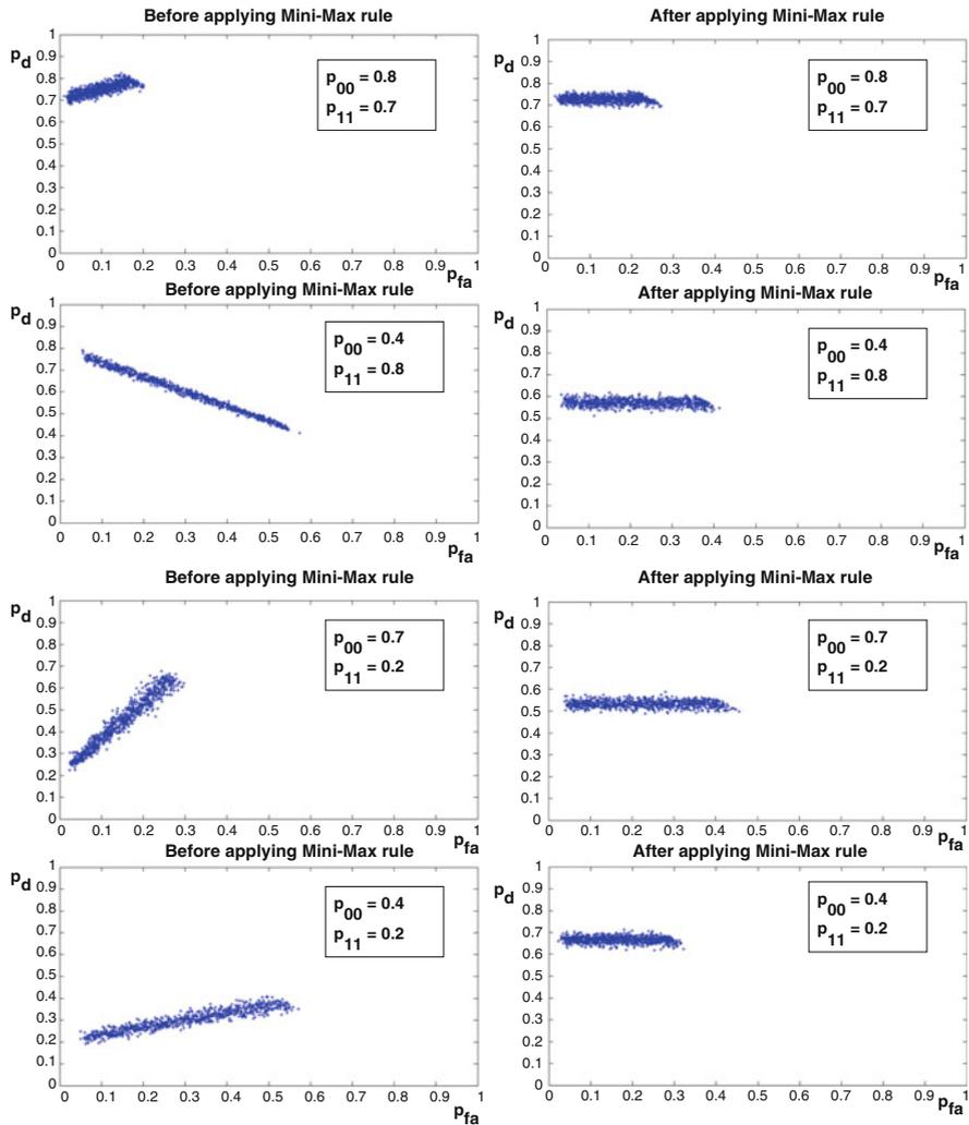
**Fig. 2.7** Illustration of mini-max rule. Subplots in the first column are obtained by receiving the bits described by the binary channel with the typical values  $p_{00} = p(0/0)$  and  $p_{11} = p(1/1)$
