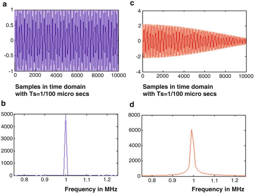
**Fig. 1.8** (a) Transmitted signal, (b) corresponding spectrum of the transmitted signal, (c) received signal after subjected to multi-path slow fading and (d) corresponding spectrum of the received signal
