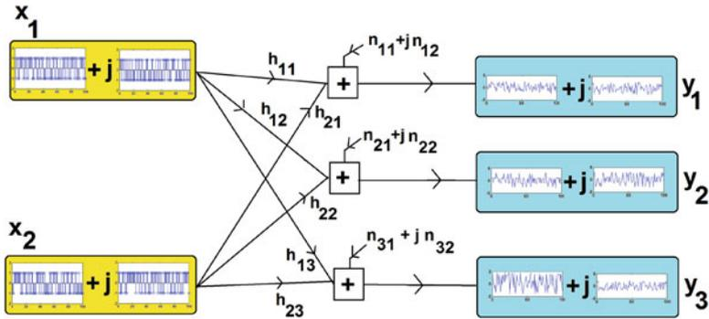
**Fig. 1.18** Illustration of MIMO with channel matrix  $G$  (complex co-efficients  $h_{11}, h_{12}, h_{13}, h_{21}, h_{22}, h_{23}$ ) and additive complex random variable,  $n_{11} + jn_{12}$ ,  $n_{21} + jn_{22}$  and  $n_{31} + jn_{32}$
