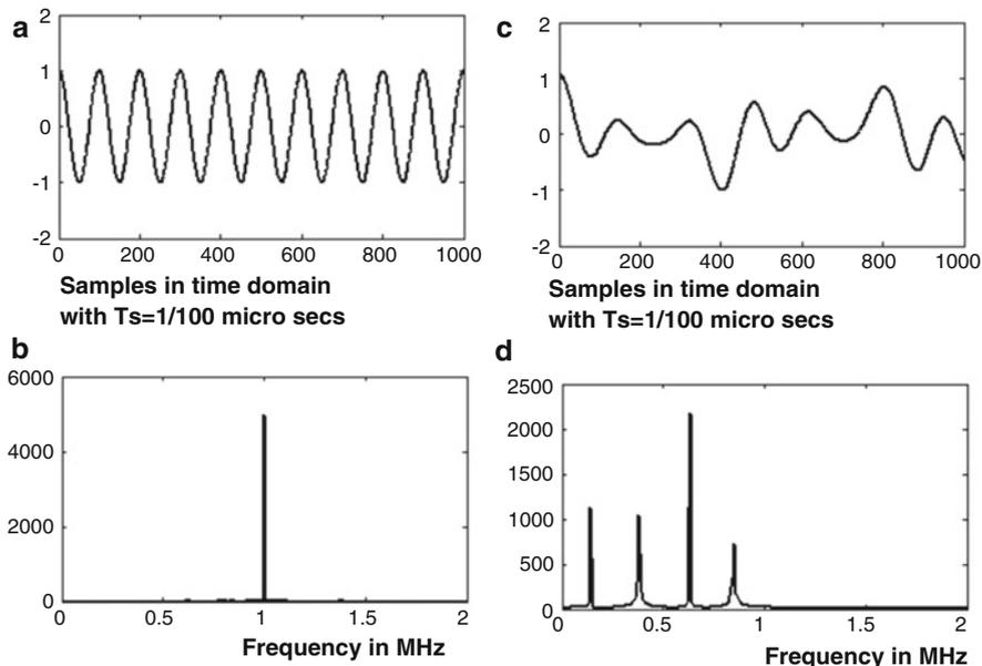
**Fig. 1.6** (a) Transmitted signal, (b) corresponding spectrum of the transmitted signal, (c) received signal after subjected to multi-path fast fading and (d) corresponding spectrum of the received signal
