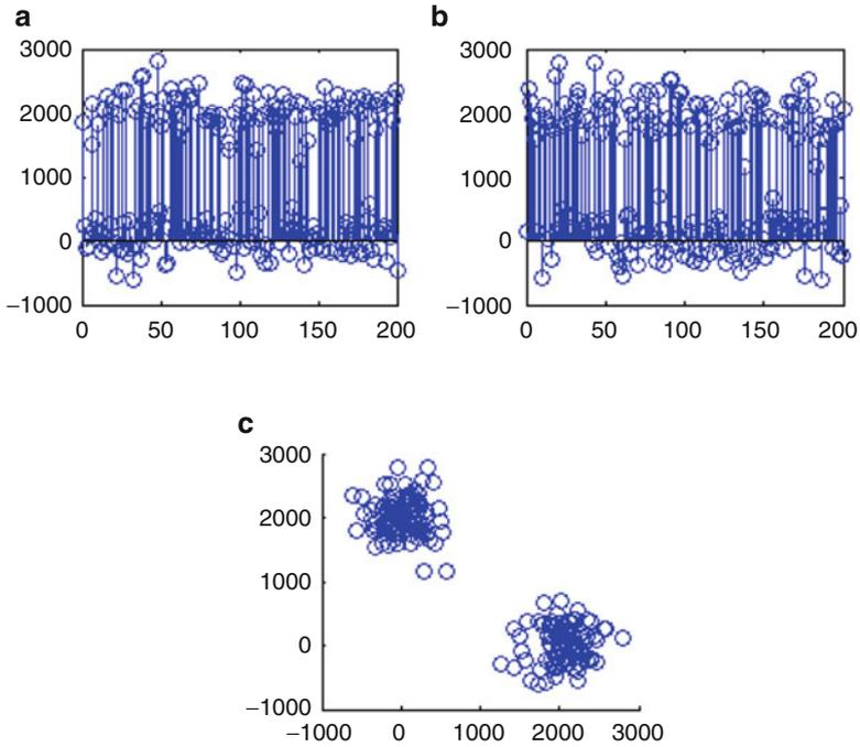
**Fig. 3.11** (a) Output of the correlation receiver 1. (b) Output of the correlation receiver 2. (c) Signal-space diagram for the FSK signal
