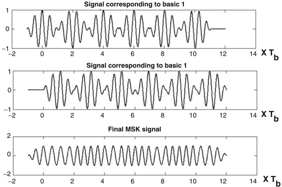
Fig. 3.15 Sample waveform of the MSK signal
