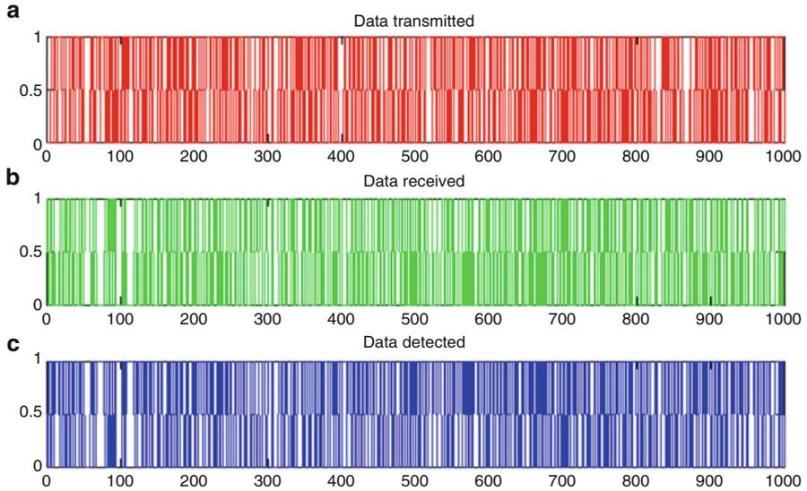
**Fig. 2.6** (a) Data transmitted, (b) Data received and (c) data detected using Bayes technique. Probability of detection and the probability of false alarm obtained are 0.8260 and 0.14, respectively, with  $p_{00} = 0.2589$  and  $p_{11} = 0.0678$  and the Bayes rule selected is 2. The data are generated with prior probability  $p_0 = 0.5$
