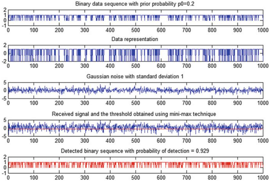
**Fig. 2.10** Illustration of mini-max rule with additive Gaussian noise channel model
