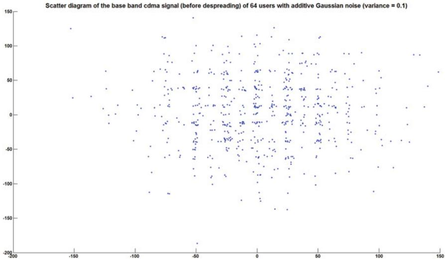
**Fig. 3.40** Scatter plot of the base band CDMA signal (64 users, with 10 instants from each user) before despreading with additive Gaussian noise (variance = 0.1)
