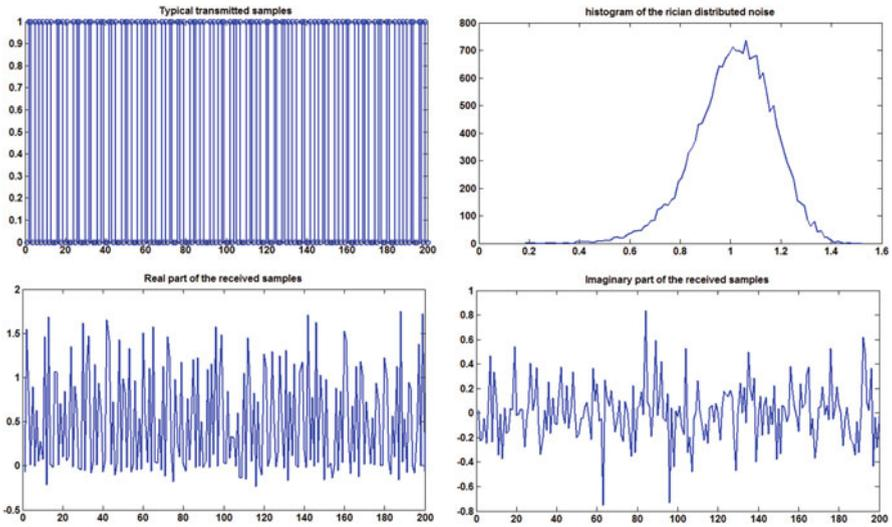
Fig. 1.15 Illustration of the Flat fading Rician model
