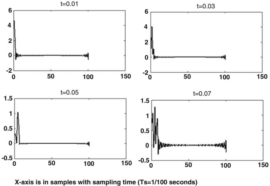
**Fig. 1.5** Zoomed version of the impulse response of the time-varying channel for the time instances  $t = 0.01$ ,  $t = 0.03$ ,  $t = 0.05$  and  $t = 0.07$
