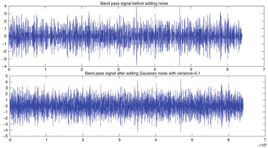
**Fig. 3.38** Typical bandpass CDMA signal for 10 symbols with 64 users
