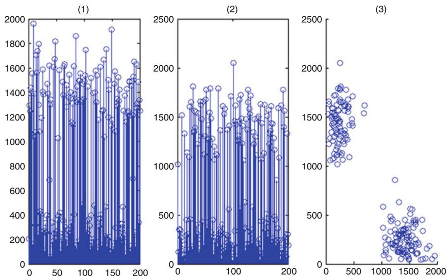
**Fig. 3.34** (a) Output of the bank of correlator receiver 1. (b) Output of the bank of correlator receiver 2. (c) Scatter diagram of the typical received FSK (detected using correlators)
