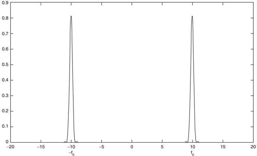
**Fig. 3.19** Spectral density of the MSK signal with  $E_b = 1\text{unit}$ ,  $T_b = 1\text{unit}$  and  $f_c = 10\text{units}$
