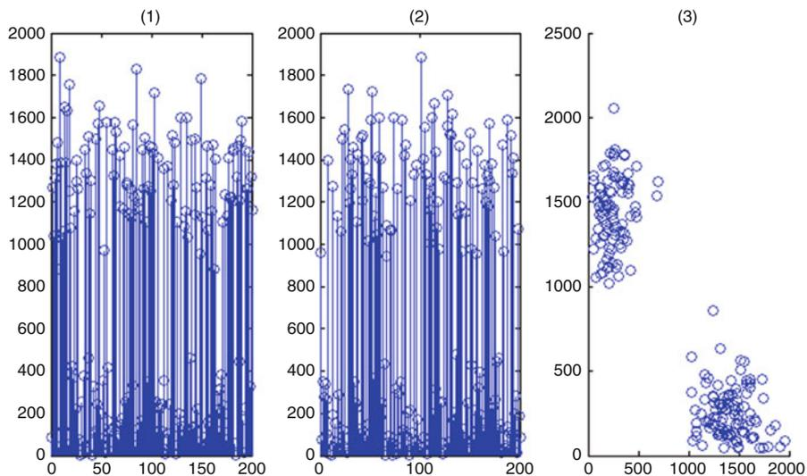
**Fig. 3.35** (a) Sampled values of the envelope detector after subjected to matched filter 1. (b) Sampled values of the envelope detector after subjected to matched filter 1. (c) Scatter diagram of the typical received FSK (detected using matched filters, followed by envelope detectors)
