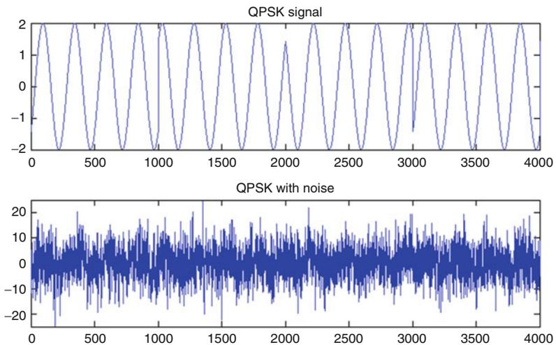
Fig. 3.21 Typical QPSK signal with noise
