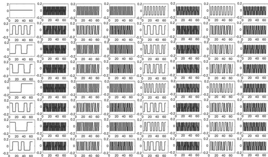
Fig. 3.37 Illustration of 64 orthogonal codes used in the CDMA
