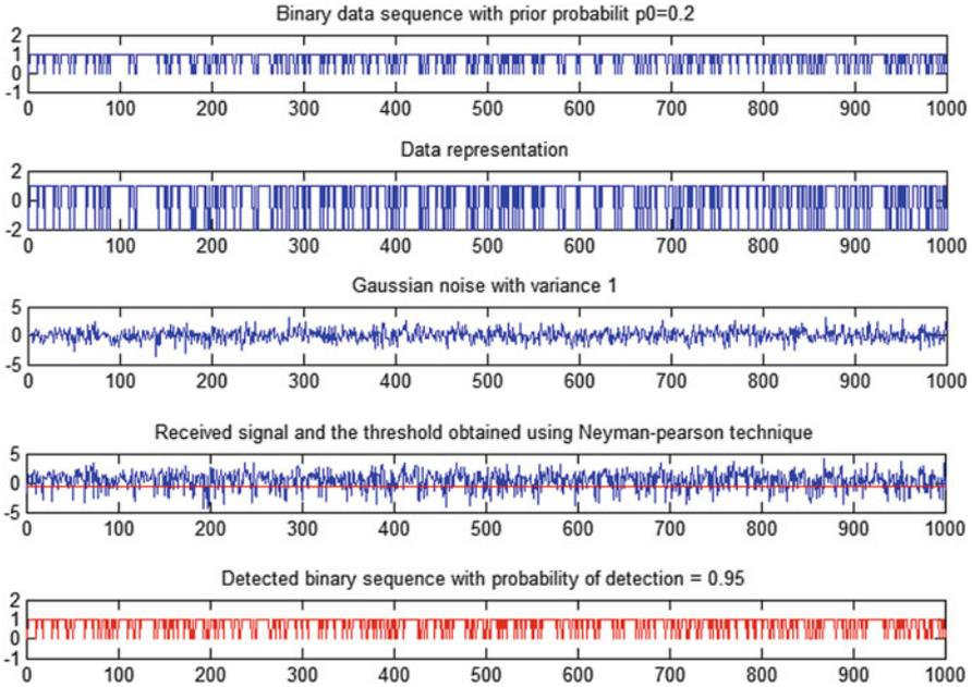
**Fig. 2.11** Illustration of Neyman–Pearson technique with additive Gaussian noise channel model with the desired probability of false alarm is 0.1
