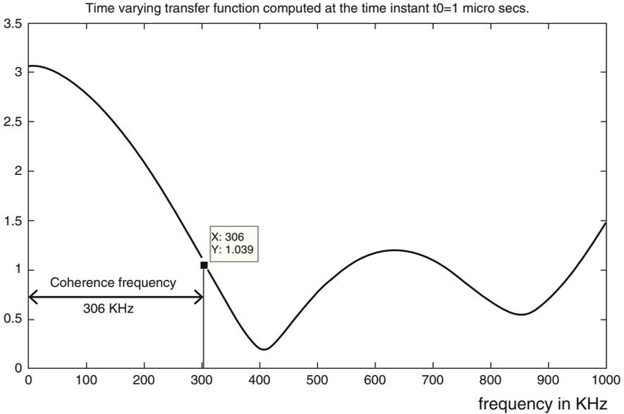
**Fig. 1.11** Illustration of the computation of the coherence frequency using delay spread ( $L$ )
