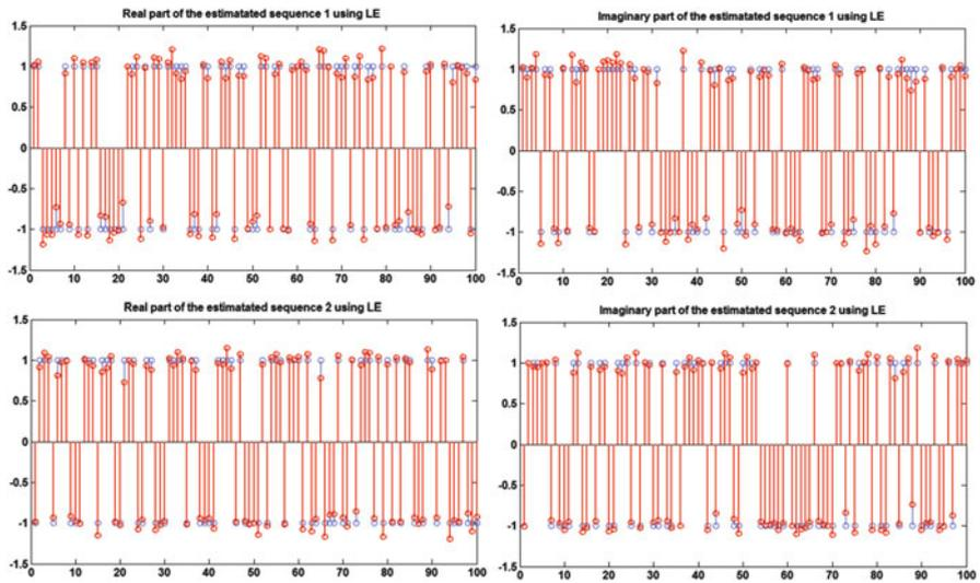
**Fig. 1.23** Linear minimum mean square estimation (MMSE) of the MIMO technique
