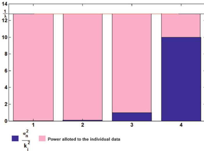
Fig. 1.31 Demonstration of water fill algorithm for power distribution in the MIMO set-up
