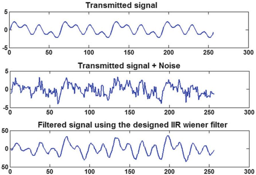
Fig. 2.16 Illustration of causal IIR Wiener filter-based estimation in time domain
