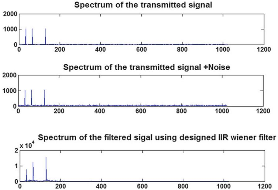
Fig. 2.17 Illustration of causal IIR Wiener filter-based estimation in frequency domain
