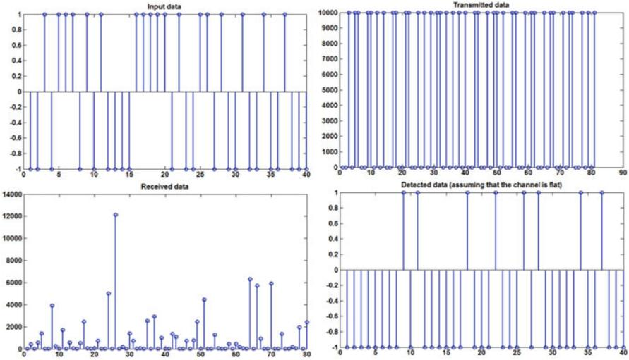
**Fig. 3.45** Demonstration of detection of binary sequence with time-varying Rayleigh channel (order 2), showing a detection rate of 75 %
