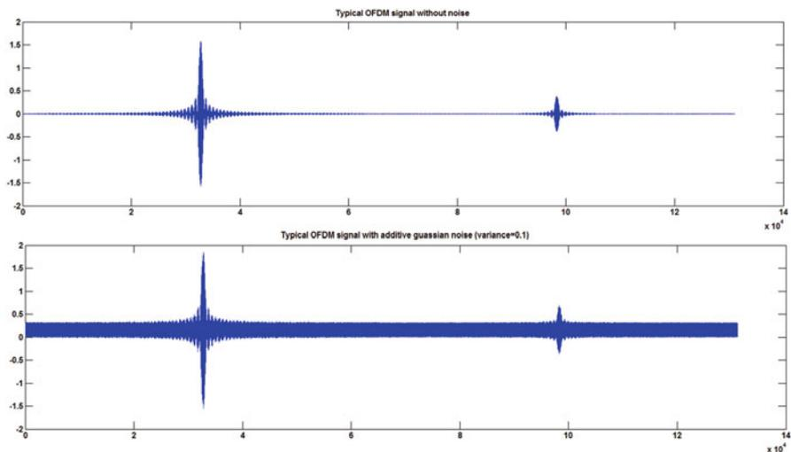
Fig. 3.29 Bandpass OFDM signal with and without additive gaussian noise
