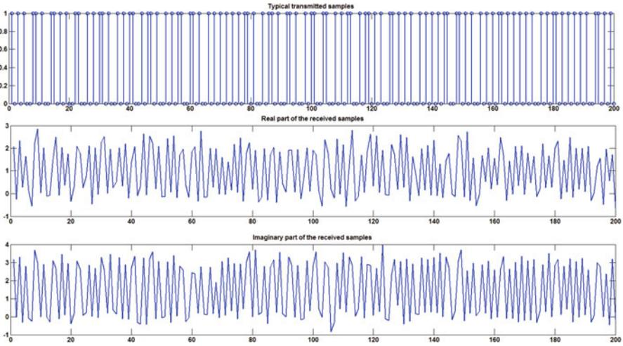
**Fig. 1.17** Illustration of the Flat channel with known estimated filter co-efficient  $2 + 3j$  and additive complex Gaussian noise (variance = 0.1)
