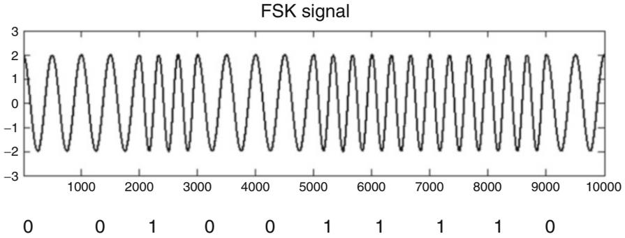
**Fig. 3.9** Typical frequency shift keying signal
