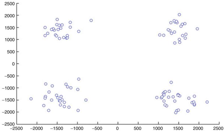
Fig. 3.23 Scatter diagram of the QPSK signal
