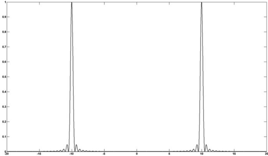
**Fig. 3.24** Spectral density of the QPSK signal with  $E_b = 1$  unit,  $T_b = 1$  unit and  $f_c = 10$  units
