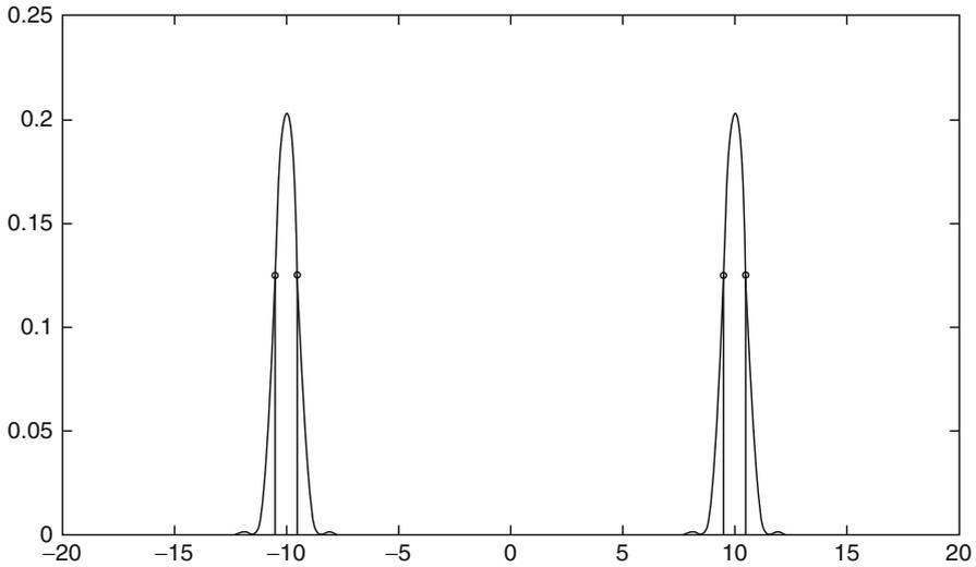
**Fig. 3.13** Spectral density of the FSK signal with  $E_b = 1$  unit,  $T_b = 1$  unit and  $f_c = 10$  units
