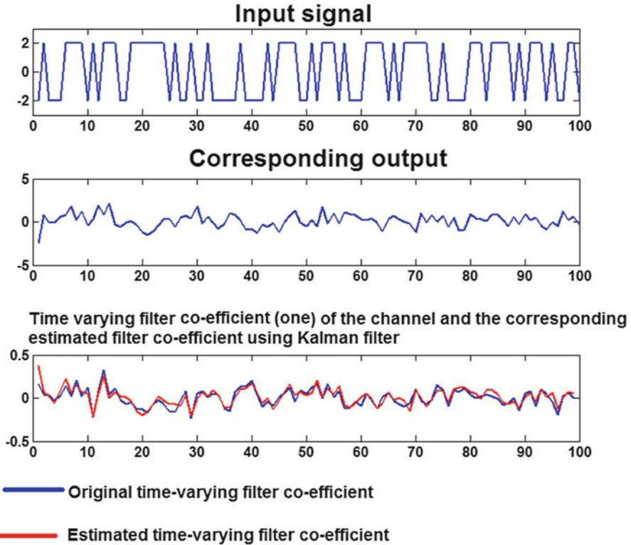
Fig. 2.18 Illustration of the kalman filter
