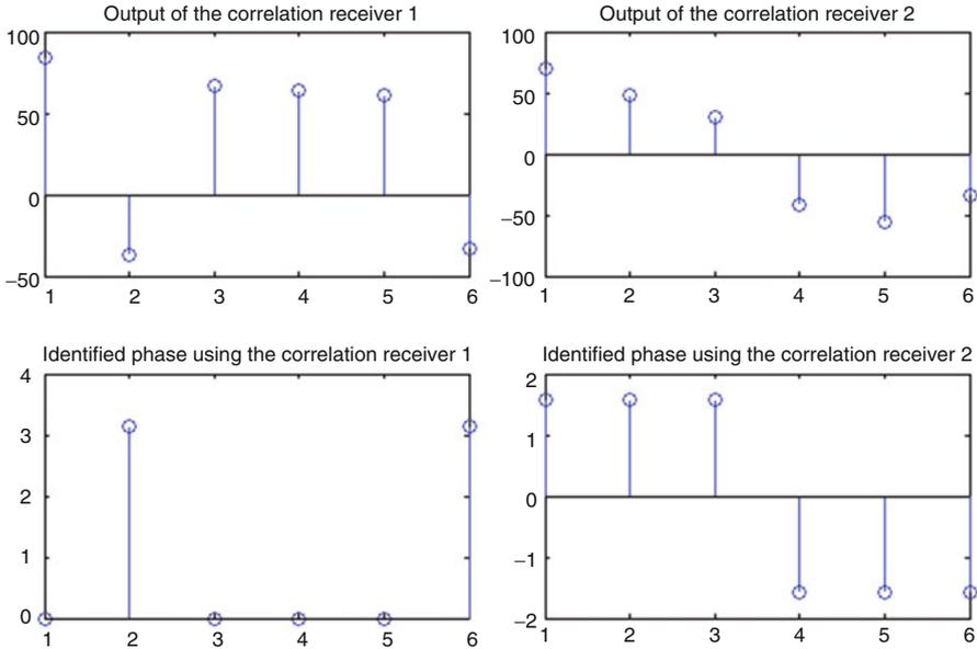
**Fig. 3.17** Illustration of the output of the correlation receiver for MSK detection
