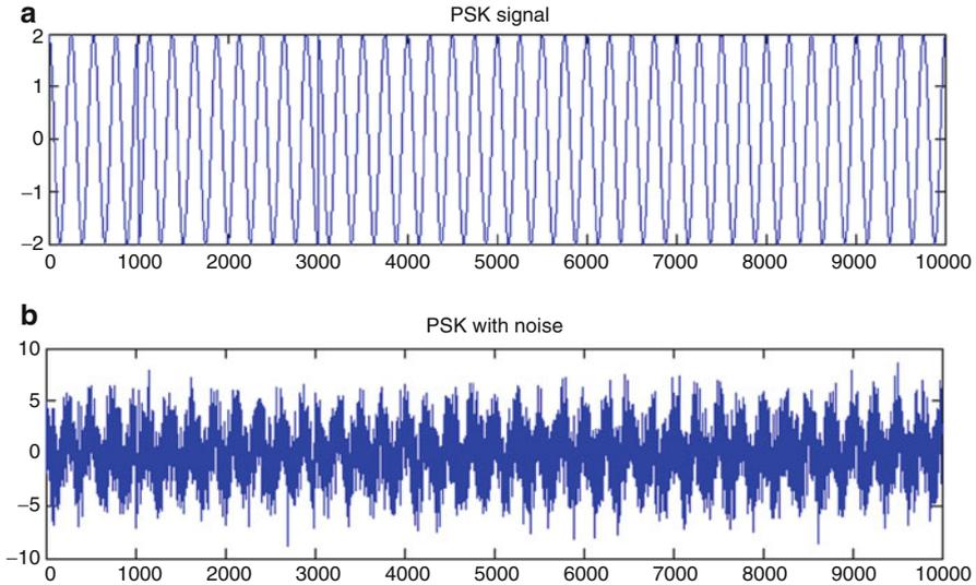
**Fig. 3.6** (a) PSK signal and (b) PSK signal with additive Gaussian noise (variance = 4)
