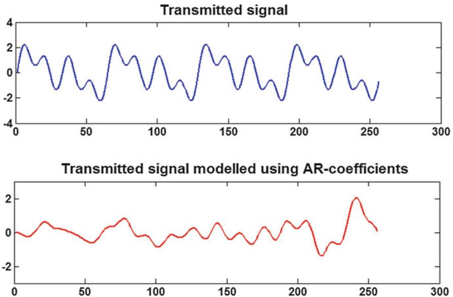
Fig. 2.15 Illustration of the AR model of the transmitted message signal
