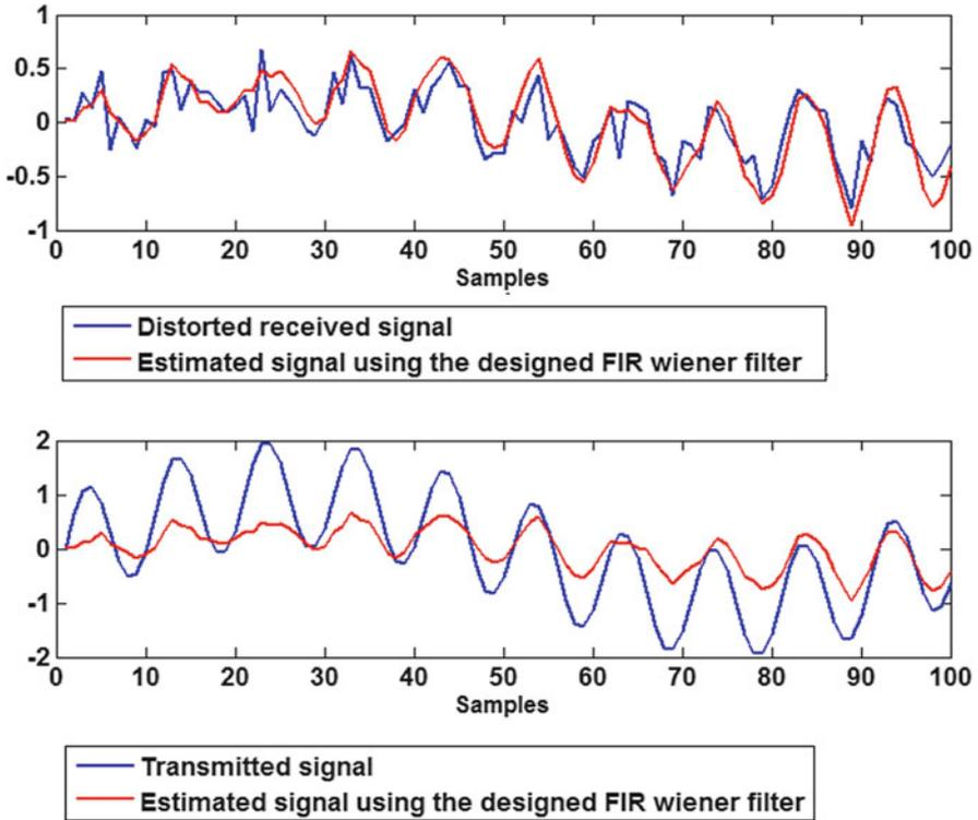
Fig. 2.13 Illustration of FIR Wiener filter-based estimation
