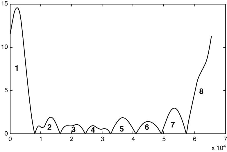
**Fig. 3.26** Illustration of the sub-band achieved using OFDM techniques (by computing the spectrum of  $C_{OFDM}^{BASEBAND}(t)$ )
