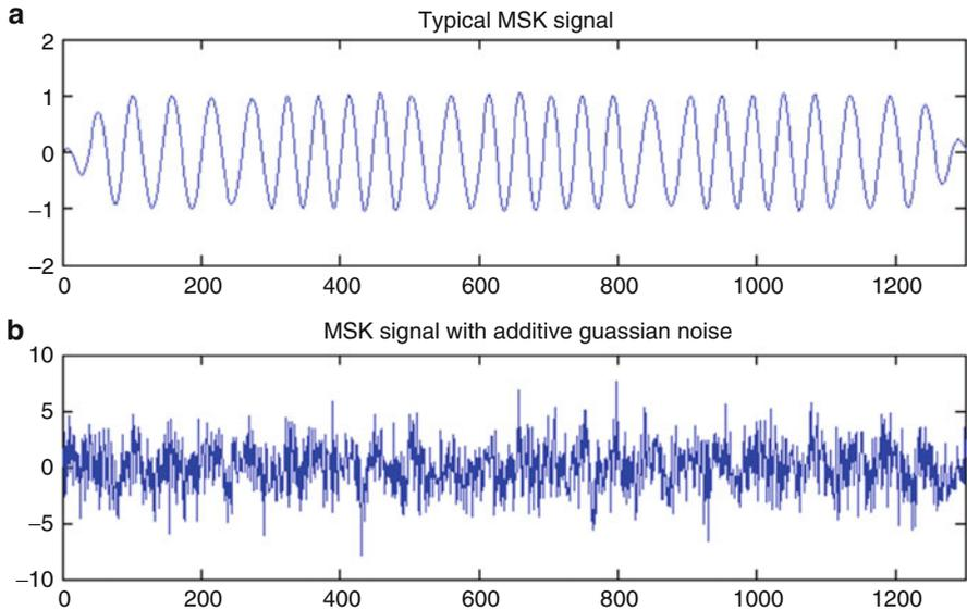
**Fig. 3.16** (a) Typical MSK signal. (b) MSK signal with additive Gaussian noise (variance = 4)
