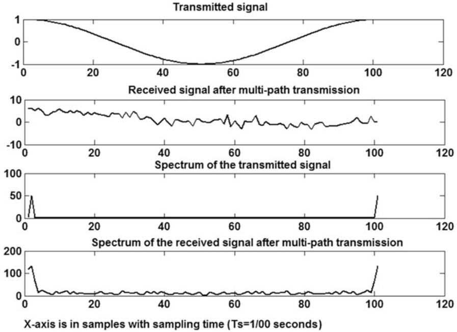
Fig. 1.1 Illustration of the multi-path transmission
