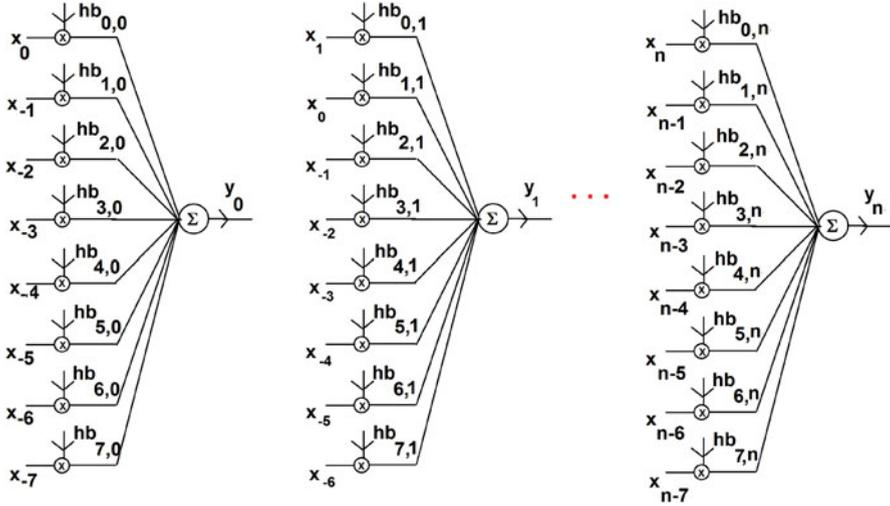
Fig. 1.12 Illustration of discrete wireless time-varying model
