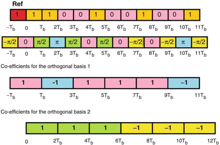
**Fig. 3.14** Illustration of the minimum shift keying
