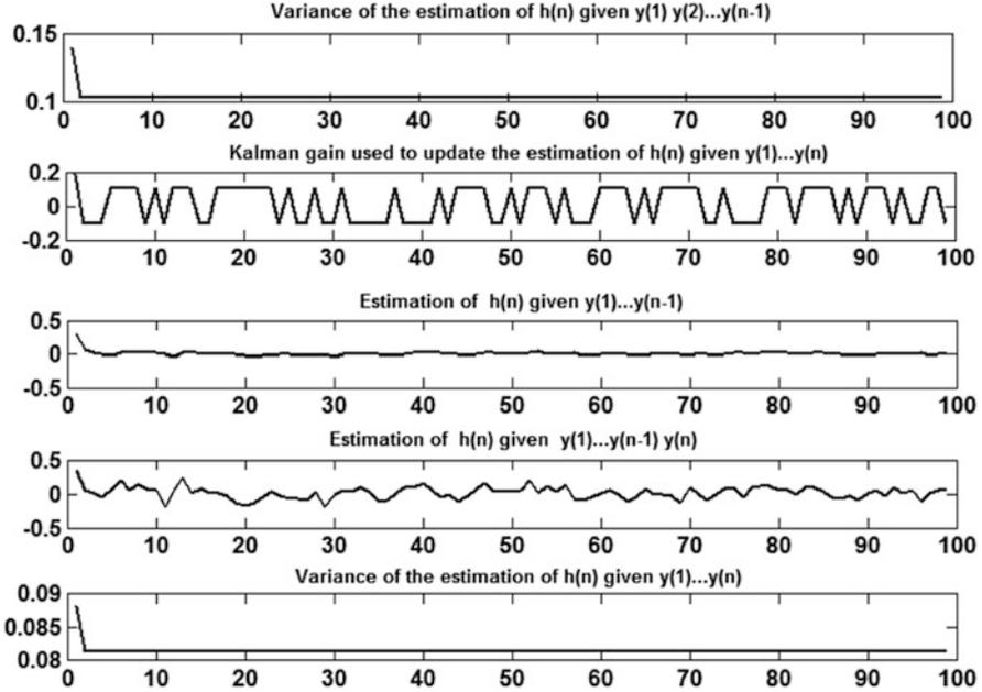
Fig. 2.19 Illustration of the kalman filter (continued)
