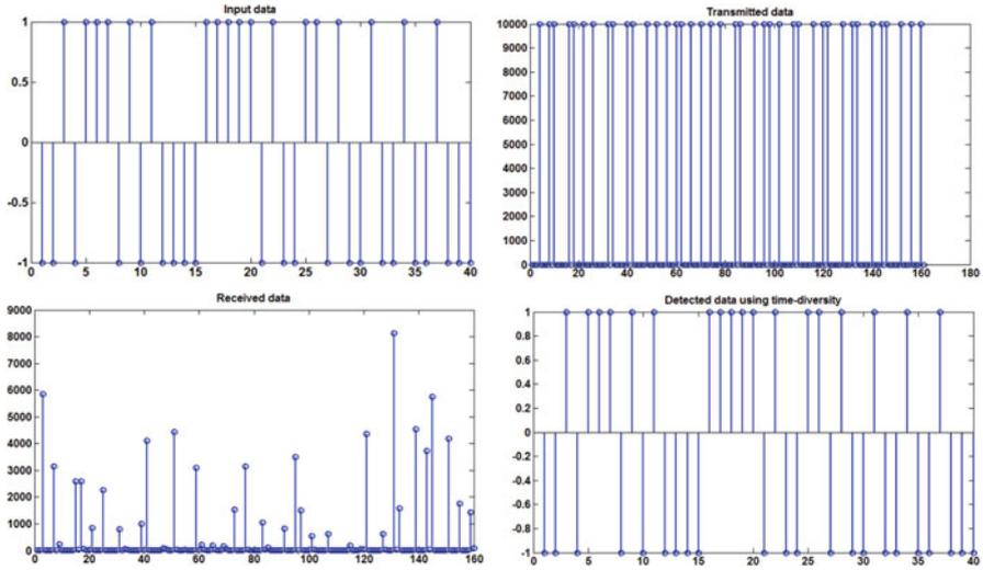
**Fig. 3.46** Demonstration of detection of binary sequence with time-varying Rayleigh channel (order 2) using time-diversity, showing a detection rate of 100 %
