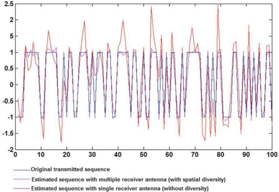
**Fig. 3.44** Demonstration of spatial diversity showing the actual and the estimated imaginary parts of the transmitted base band sequence
