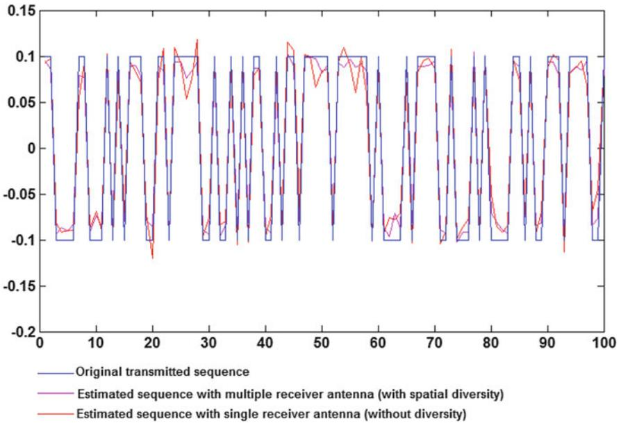
**Fig. 3.43** Demonstration of spatial diversity showing the actual and the estimated real parts of the transmitted base band sequence
