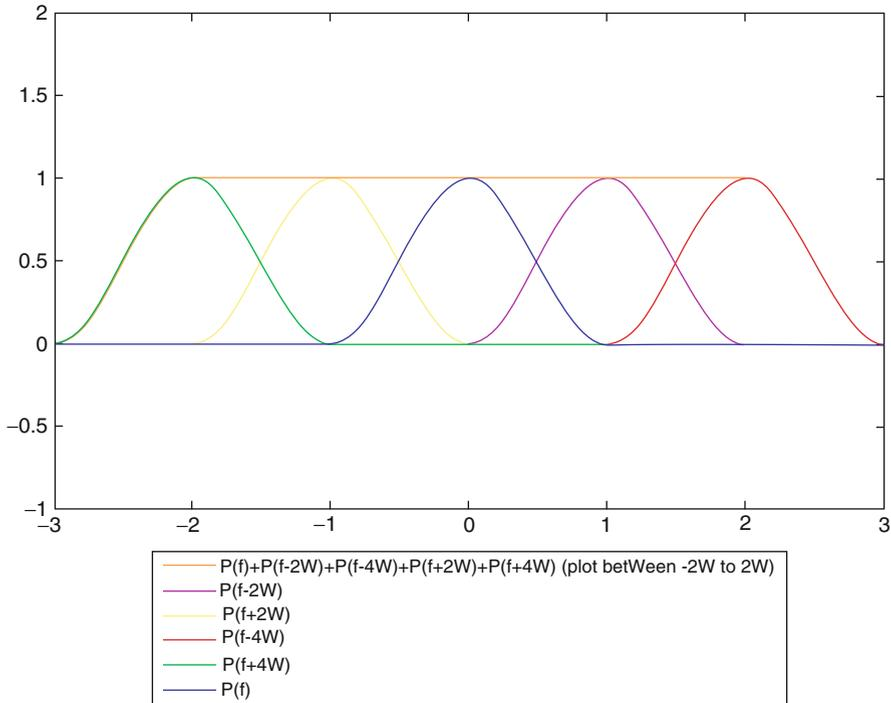
**Fig. 3.3** Illustration that for the modified pulse  $P_{\text{mod}}(f)$  with  $\alpha = 1$ ,  $P_{\text{mod}}(f) + P_{\text{mod}}(f - 2W) + P_{\text{mod}}(f - 4W) + P_{\text{mod}}(f + 2W) + P_{\text{mod}}(f + 4W) = 1$  for  $-3W \leq f \leq 3W$ . This illustrates that the modified pulse satisfies (3.16)
