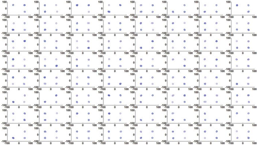
**Fig. 3.41** Scatter plot of the detected base band for 64 users (with 10 samples from each user) after despreading. Less than four clusters in some of the subplots implies that the corresponding user data do not have all the four varieties
