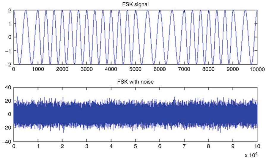
**Fig. 3.10** (a) FSK signal. (b) FSK signal with additive Gaussian noise (variance = 4)
