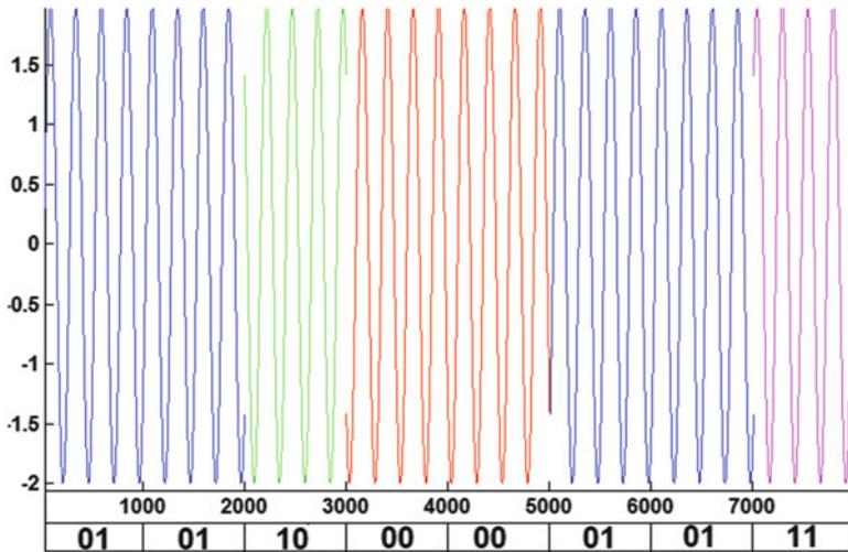
Fig. 3.20 Illustration of the typical QPSK signal
