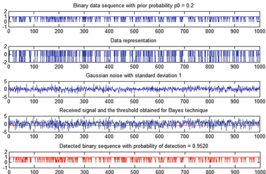
Fig. 2.9 Illustration of Bayes rule with additive Gaussian noise channel model
