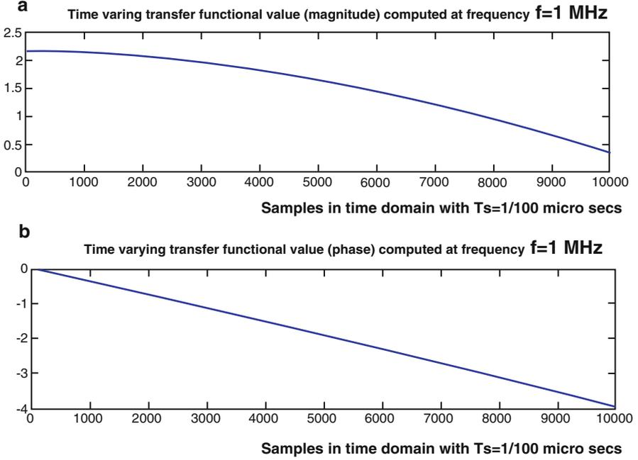
**Fig. 1.9** Illustration of the slow fading channel characteristics
