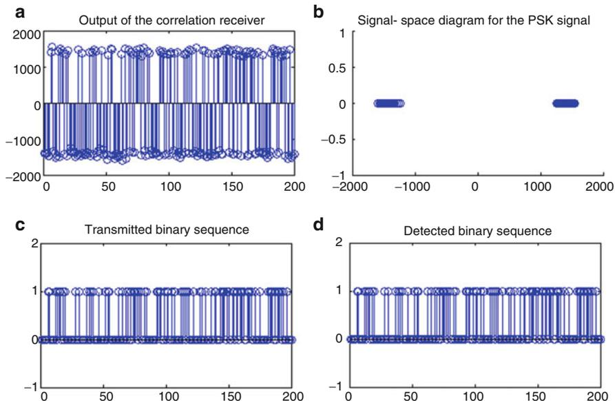
Fig. 3.7 Demonstration of the PSK signal detection using the correlation receiver
