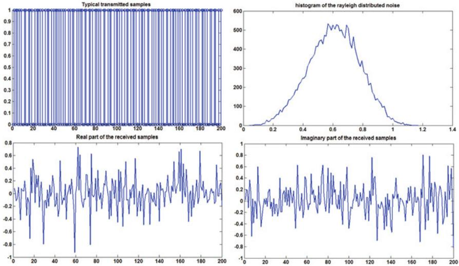
**Fig. 1.13** Illustration of the flat fading Rayleigh model
