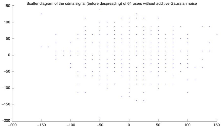
**Fig. 3.39** Scatter plot of the base band CDMA signal (64 users) before despreading without additive Gaussian noise
