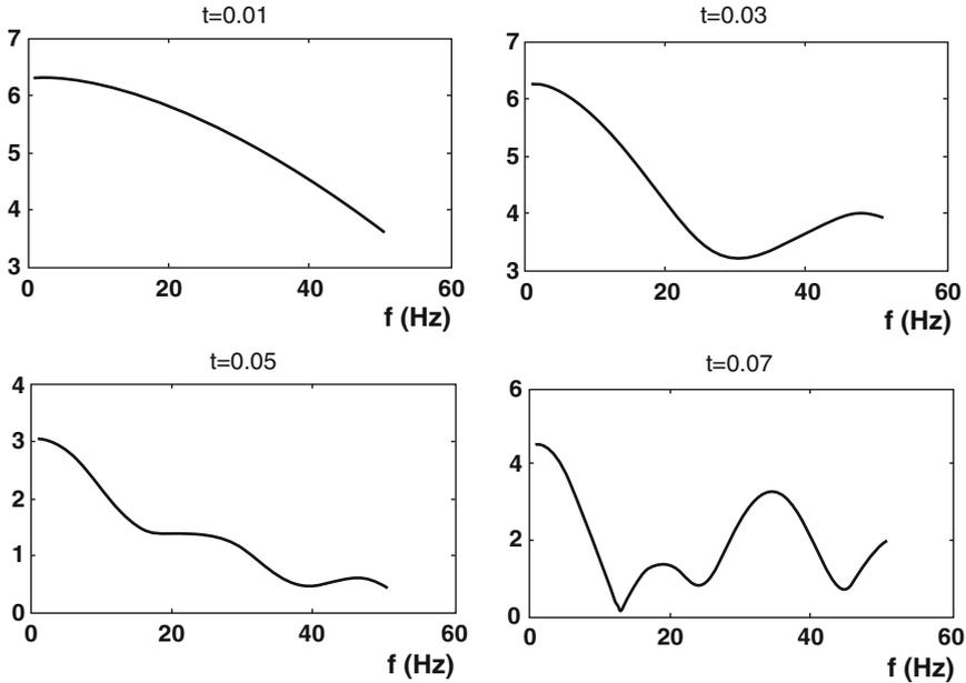
**Fig. 1.3** Zoomed version of the transfer function of the time-varying channel for the time instances  $t = 0.01$ ,  $t = 0.03$ ,  $t = 0.05$  and  $t = 0.07$
