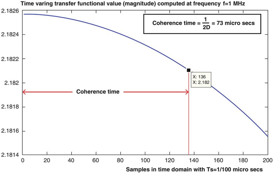
**Fig. 1.10** Illustration of the computation of the coherence time using Doppler spread ( $D$ )
