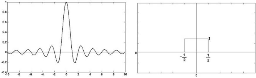
**Fig. 3.1** (a) Truncated Nyquist pulse in time domain with  $T_b = 1$ ; (b) Nyquist pulse in frequency domain with  $W = 1/2$
