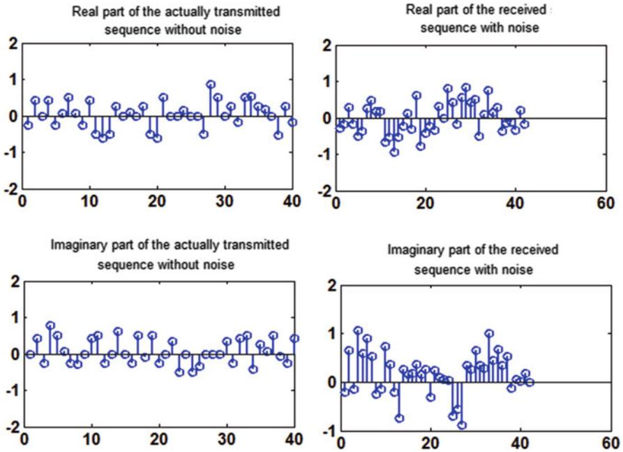
Fig. 3.31 Typical discrete transmitted OFDM signal with and without additive noise
