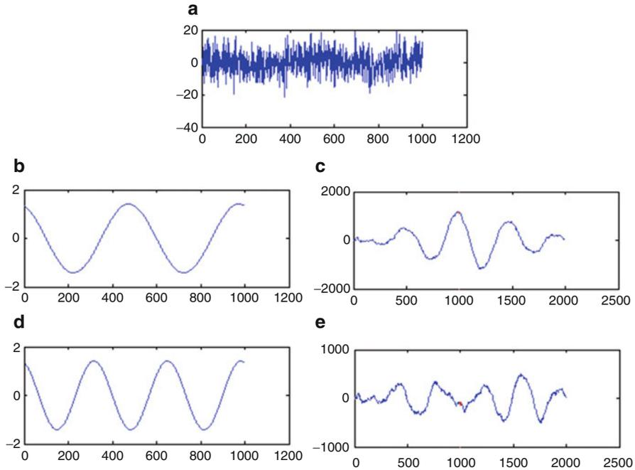
**Fig. 3.33** (a) Received noisy FSK signal corresponding to symbol 0. (b) Impulse response of the matched filter 1 (corresponding to symbol 0). (c) Output of the matched filter 1. (d) Impulse response of the matched filter 2 (corresponding to symbol 1). (e) Output of the matched filter 2
