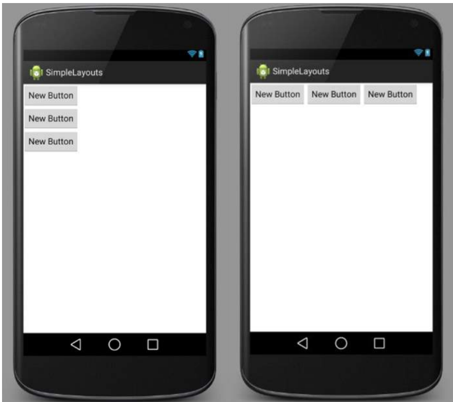
Figure 8-8. Vertical LinearLayout vs. a Horizontal LinearLayout
