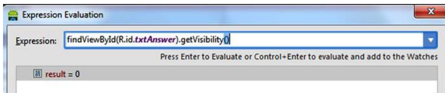
Figure 12-8. Examine the answer EditText 's visibility in the Evaluate Expression dialog box
