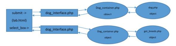
Figure 4-5. Data flow for the dog application
