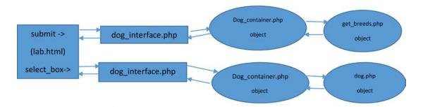
*Figure 5-1. Data flow for the dog application*
