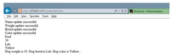
Figure 3-4. Dog class output with set and get methods
