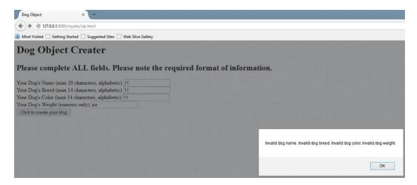
Figure 4-3. The lab.html file after failing JavaScript verification
