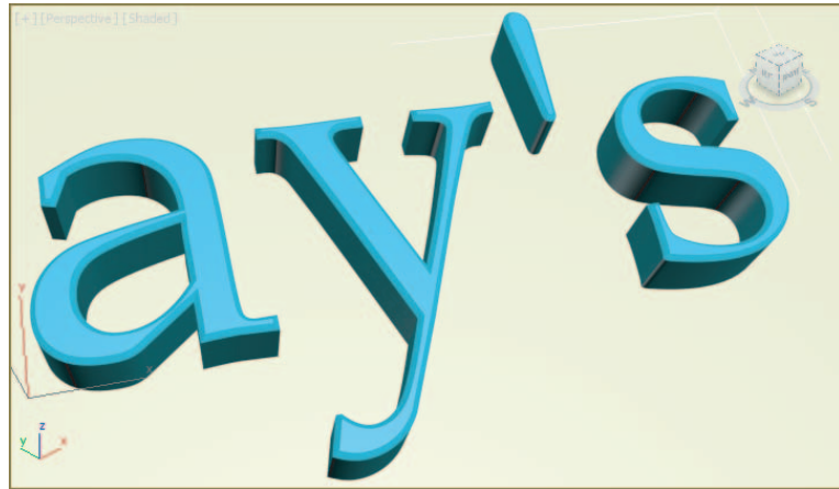
FIGURE 3.87 The chamfered effect of the Bevel modifier
