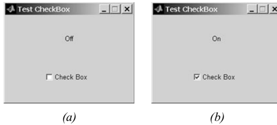
Figure 10.19 (a) The GUI produced by program test_checkbox when the toggle button is off. (b) The GUI when the toggle button is on.
