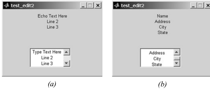
Figure 10.15 (a) The GUI produced by program test_edit2 . (b) The GUI after a user types four lines into the edit box and presses ESC.
