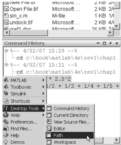
Figure 1.4 The Start Button, which allows a user to select from a wide variety of MATLAB and desktop tools.
