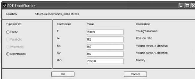
Figure 13.39 PDF specification for input of the materials constants and density. (From MATLAB. With permission.)
