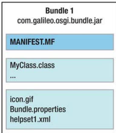
Figure 4-1. Components of an OSGi bundle
