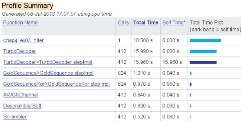
Figure 4.5 Profiling results for a system model, showing the turbo decoder to be the bottleneck
