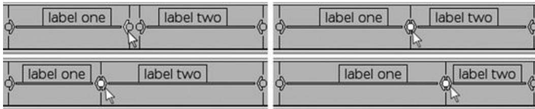
Figure 9-10. Circle handles move the whole label, and angle handles create and resize region labels. You can join region label borders and then move the border with the circle handle, and you can separate them with the angle handles.
