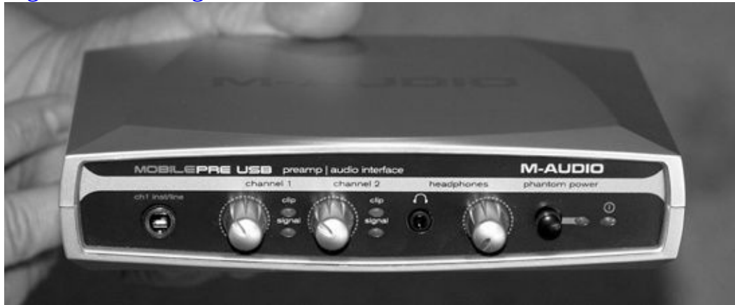
Figure 2-3. M-Audio MobilePre, front. From left to right: Channel 1 1/4" mono TRS jack, Ch. 1 and 2 gain controls, clip LEDs, headphone port, headphone volume knob, phantom power switch, phantom power LED, and power LED
