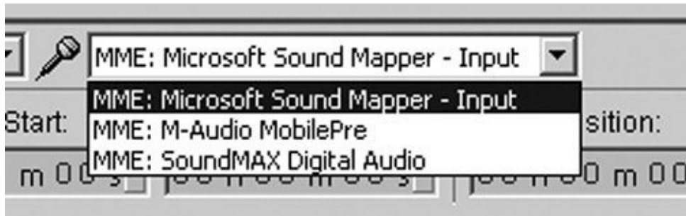
Figure 14-8. Recording device picker on Windows XP—don’t choose Microsoft Sound Mapper
