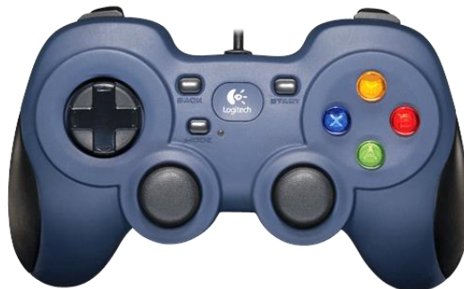
Figure 6 – The colored buttons on the right side of the gamepad will be used to control servo position.
