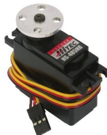
Figure 4 – An example of a servo motor that is commonly used on FIRST Tech Challenge robots. 4
