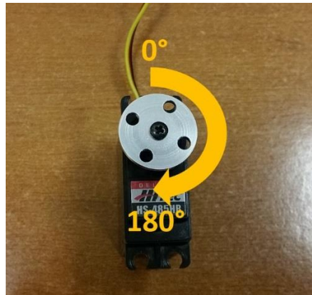
Figure 5 - A typical servo motor can rotate to and hold a position from 0 to 180 degrees.
