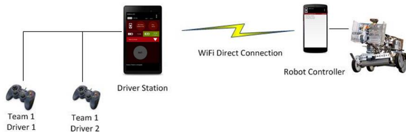
Figure 1 – The control system has a Driver Station connected wirelessly to a Robot Controller.
