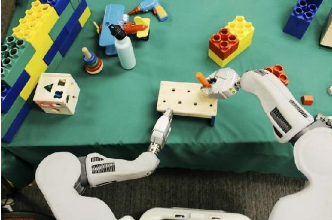
USING DEEP LEARNING , the Berkeley Robot for the Elimination of Tedious Tasks (Brett) places a peg in a hole at the University of California, Berkeley.
