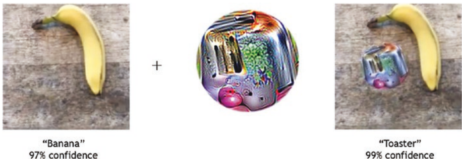
Figure 4-10. The addition of an adversarial patch to a scene with a banana is able to trick the model into falsely labeling it as a toaster
