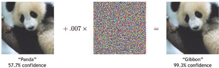
Figure 4-9. A small change that is imperceptible to humans can cause a machine learning model to confidently output the wrong label
