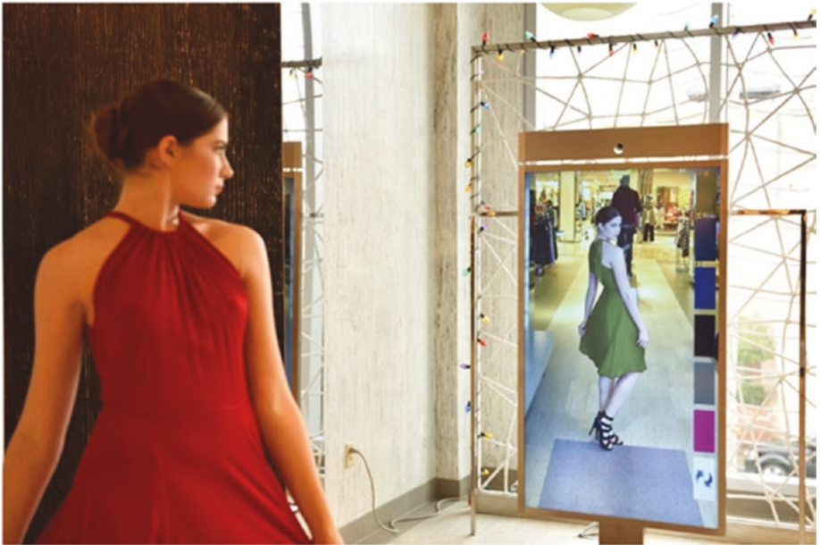
Figure 3-1. A woman trying on a dress using MemoMi's smart mirror with augmented reality features to change the color of the garment in real time
