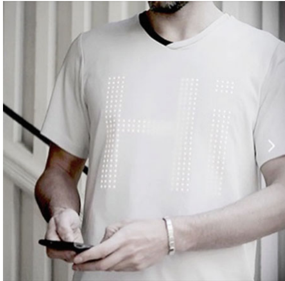
Fig. 1 LED-embedded shirt provides an illuminative graphics display
