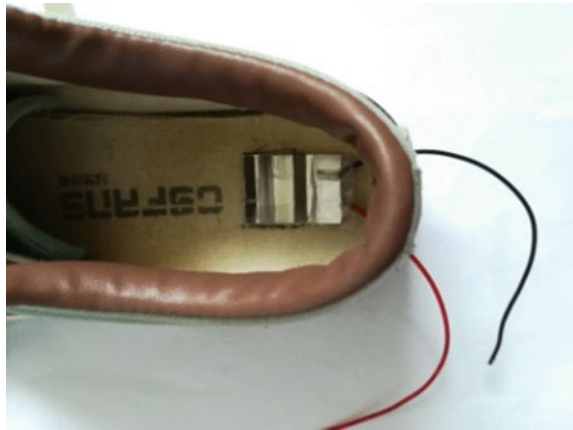
Fig. 2 Scheme of the simple force excitation generator. a Structure; b Schematic
