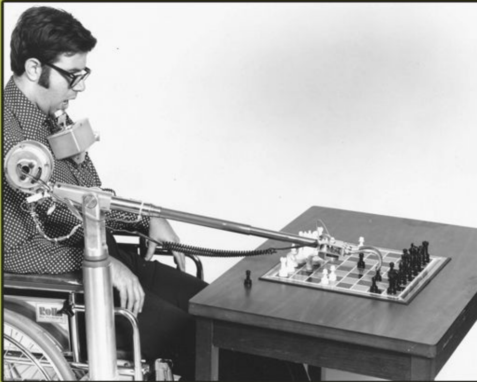
This robot arm wheelchair is operated by the pressure of the handicapped person's chin. The gripper hand can do all kinds of tasks, including moving chess pieces. (Veteran's Administration)
