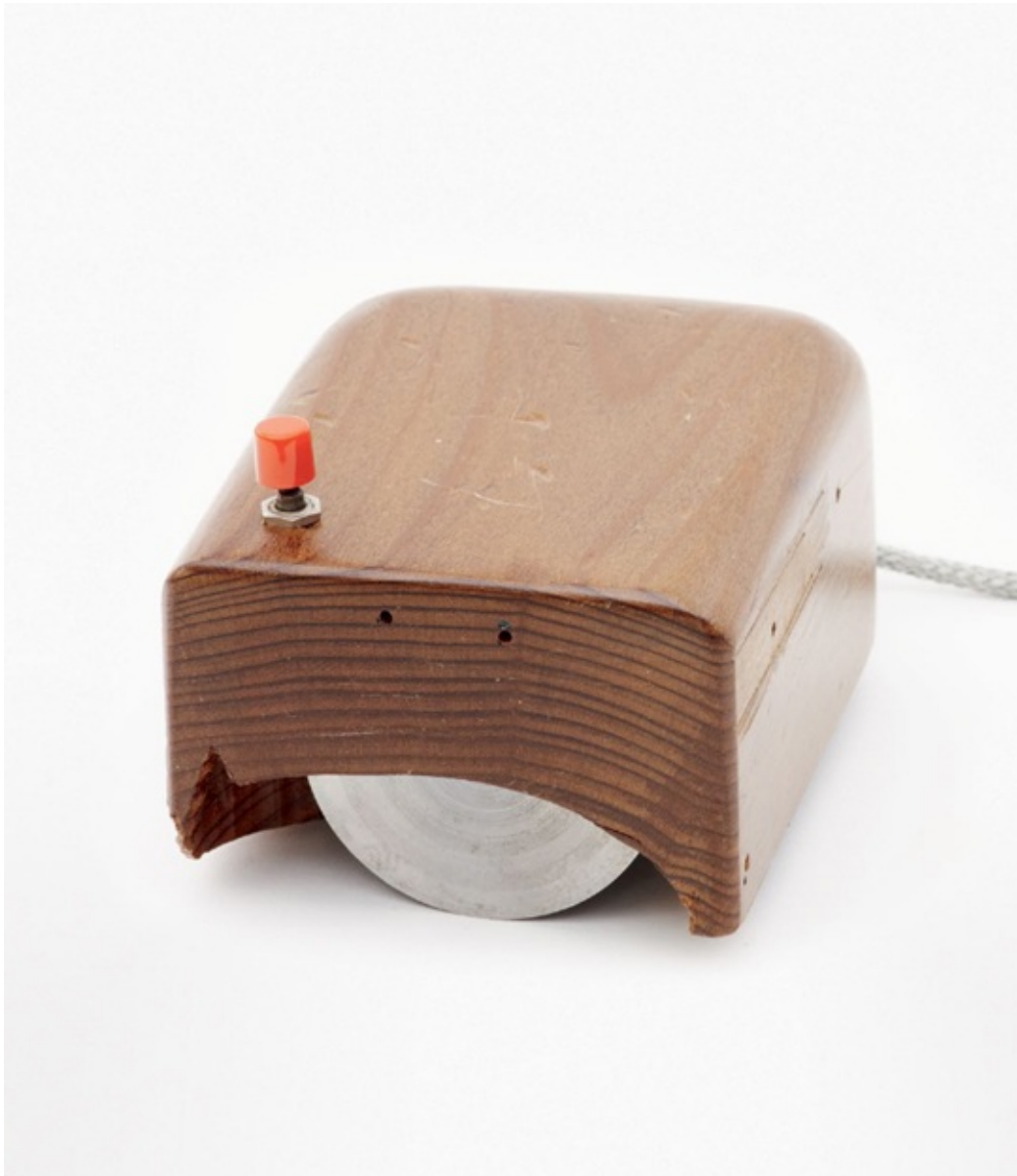
Replica of Engelbart's mouse prototype, built by engineer Bill English, 1964.
