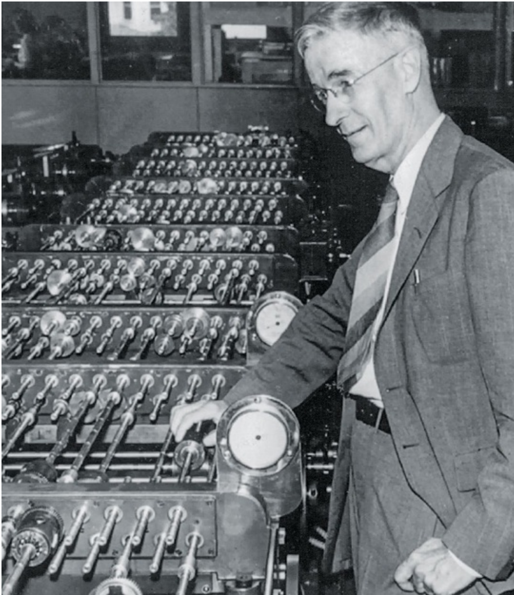
Vannevar Bush with his differential analyzer, a mechanical computer designed to solve differential equations.
