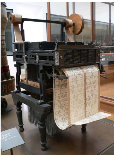
Figure 2.13. Reconstruction of a Jacquard loom.
