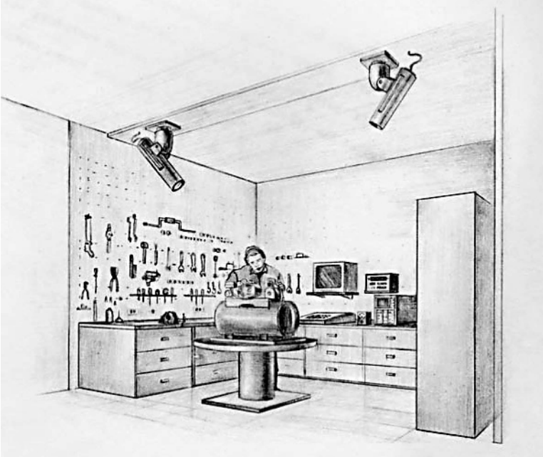
Figure 18.1. Proposed arrangement for helping an apprentice. (Used with permission of SRI International.)
