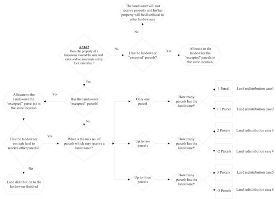
Fig. 8.1 The main decision tree for the design module of LandSpaCES
