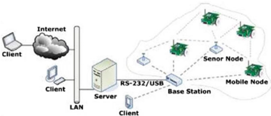
Fig. 8 The system architecture of a MSN [26]
