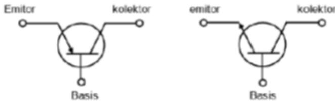
Gambar 3. 3 Simbol Transistor
