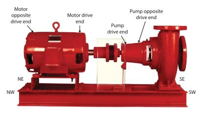
**Figure 10.1** Identifying vibration measurement locations.
