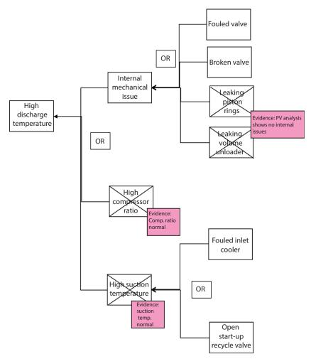
Figure 11.2 Reciprocating compressor fault tree.
