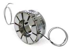
**Figure 17.2** Thrust bearing with multiple embedded thermocouples.
