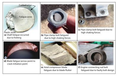
Figure 3.3 Fatigue failures.
