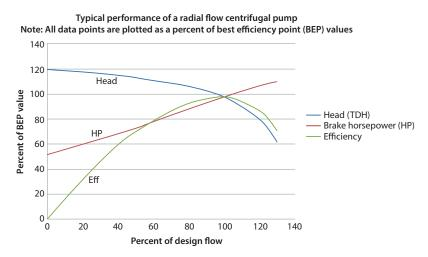
Figure A.1 Radial flow pump.
