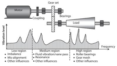
Figure 15.4 Spectrum for a complex machine.
