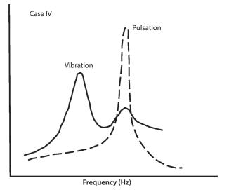
**Figure 9.10** Plotting vibration and pulsation data together to differentiate between vibration and pulsation resonances.
