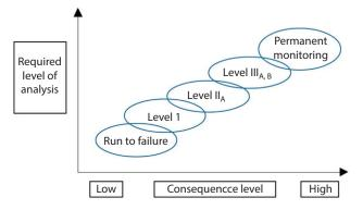
**Figure 17.3** Vibration Analysis Hierarchy. Note A—If a potential failure is detected, take additional data or get a second opinion before making a decision to repair. Note B—Employ multiple condition monitoring technologies to improve the chances of detecting early failures, such as embedded thermocouples, temporary case mounted accelerometers, ultrasonic probes, etc.
