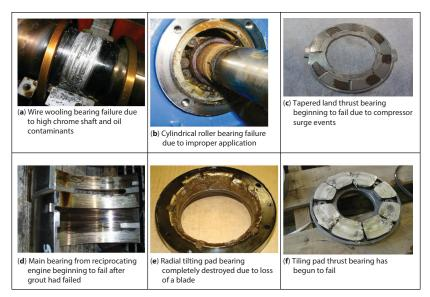
Figure 3.5 Bearing failure examples.
