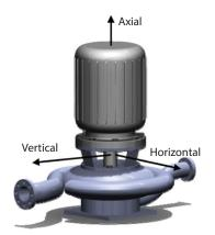
**Figure 15.1** Vibration measurement positions for an inline pump.
