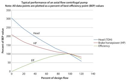
Figure A.3 Axial flow pump.
