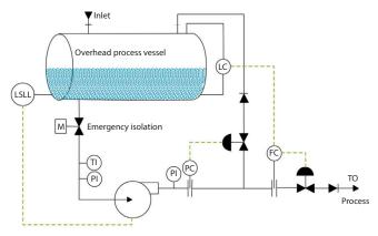
Figure 4.1 Centrifugal pumping system.
