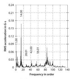
Figure 15.3 Typical vibration spectrum.
