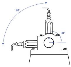
**Figure 15.7** Vibration sensors oriented 90 degrees from one another.
