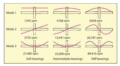
**Figure 16.1** Rotor modes shapes versus bearing stiffness.
