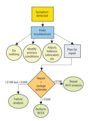
**Figure 1.1** Troubleshooting Decision Tree. Note: The dollar amounts shown here are based on the experiences of the authors. Each site may have its own trigger levels for repair costs. It goes without saying that these trigger levels need to be periodically modified for inflation.
