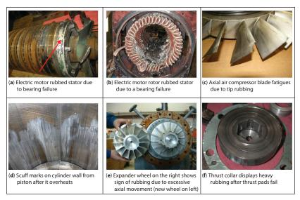
Figure 3.6 Failure resulting from rubbing examples.
