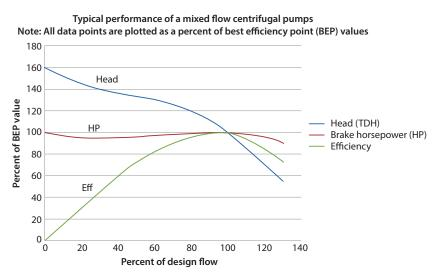
Figure A.2 Mixed flow pump.
