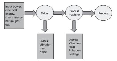
Figure 2.1 Machine energy losses.
