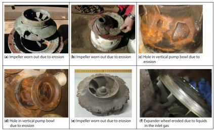
Figure 3.2 Examples of erosive wear failures.
