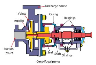
Figure 2.2 Centrifugal pump internal components.
