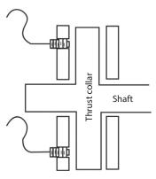
**Figure 17.1** Thrust bearing position monitored by dual thrust probes.
