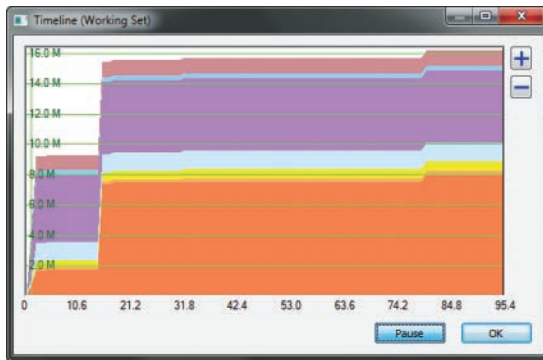
FIGURE 22-6 VMMAP timeline, clicking the “100x 1st chance” button at about the 15-second and 80-second marks.
