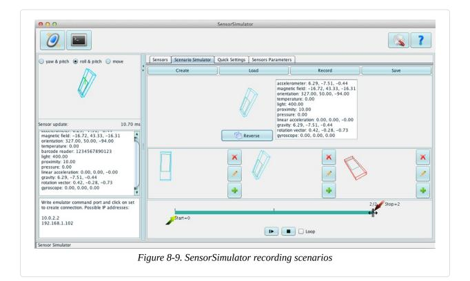
It is worth mentioning that you can record sensor interactions on a physical device. For complex scenarios, this is a simple way to record a series of UI actions that you can play back in the simulator later. Install and run an app on your device (*SensorRecordFromDevice.apk*, available in the *bin* directory) that allows you to record sensor activities. You can then play back the recorded scenario using the desktop application in the same manner as if it were created
