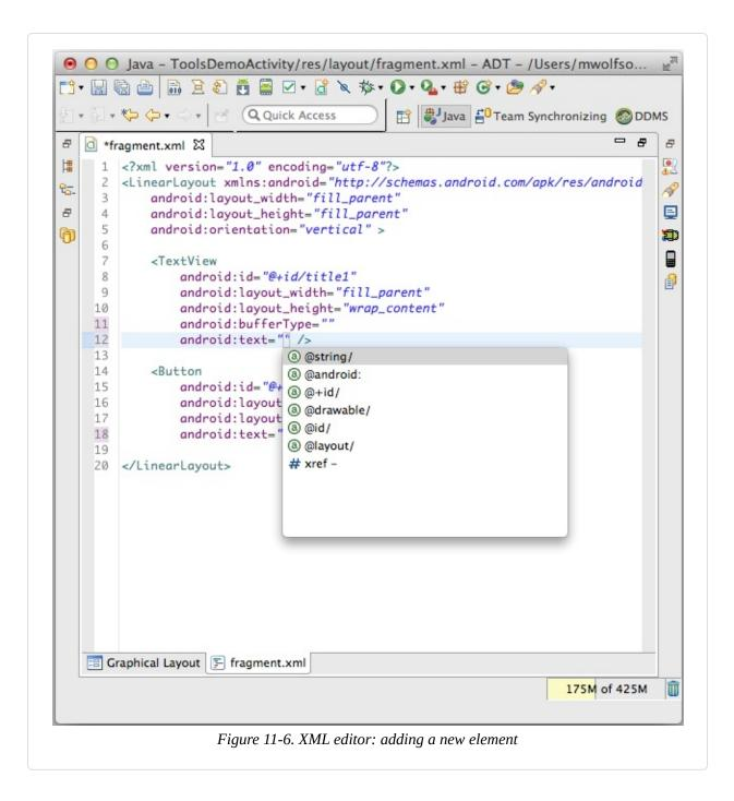
The second allows you to locate local or system resources for your UI. These things might include color definitions, string values, style definitions, or other layout elements. The example in Figure 11-7 shows how the tool provides you with a list of values available.
