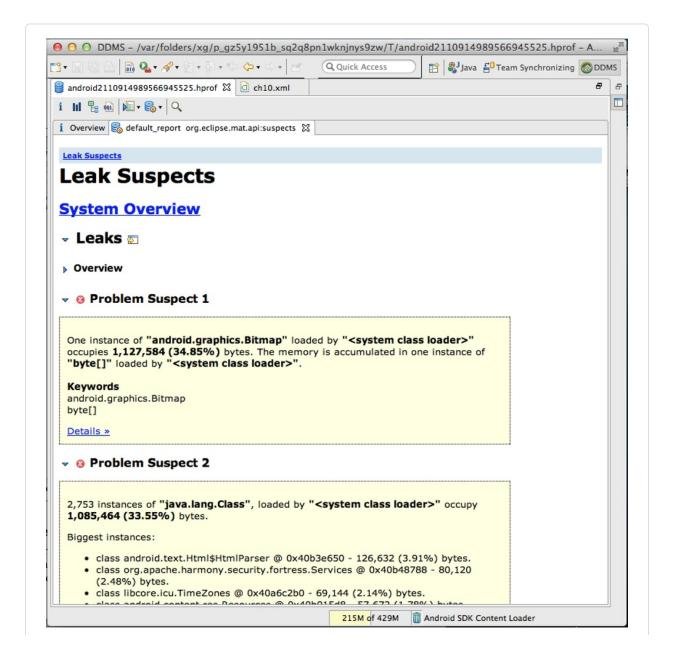
Figure 10-8. MAT Leak Suspects Report
