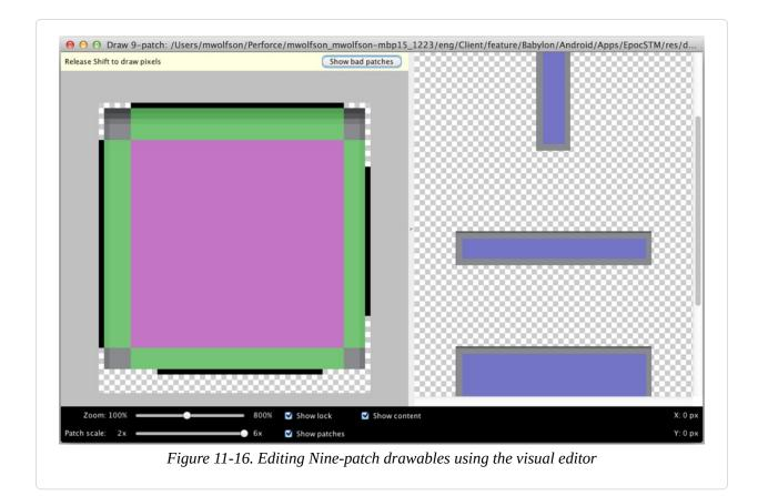
Then use the mouse to draw the lines that specify the various regions. Check the "Show patches" and "Show content" options at the bottom of the screen to visualize exactly how the system will scale your image. You can change the black lines to show:
