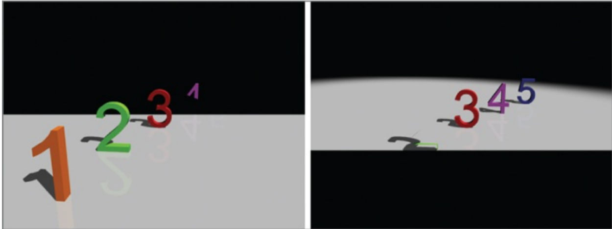
Figure 14.10 A far clipping plane cuts off the distant extents of a scene (left). A near clipping plane cuts off the extents directly in front of a camera (right).
