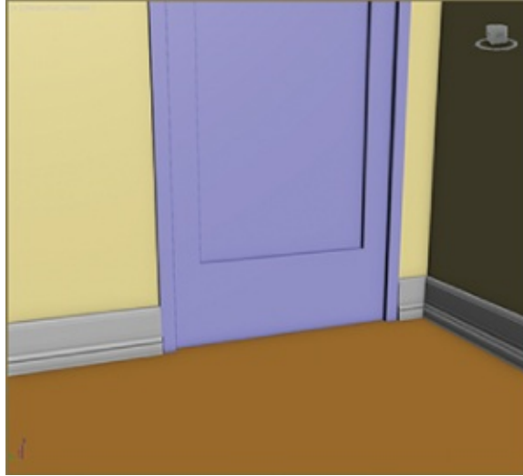
Figure 3.26 The baseboard with proper gaps at the doors
