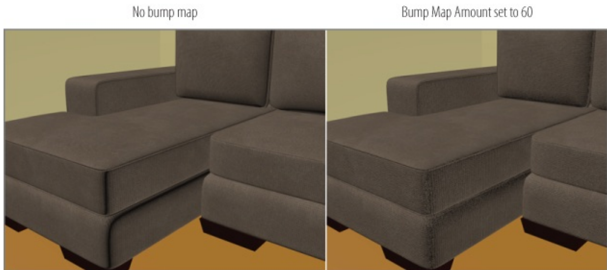
Figure 9.13 The couch fabric without the bump map (left) and with the bump map (right)
