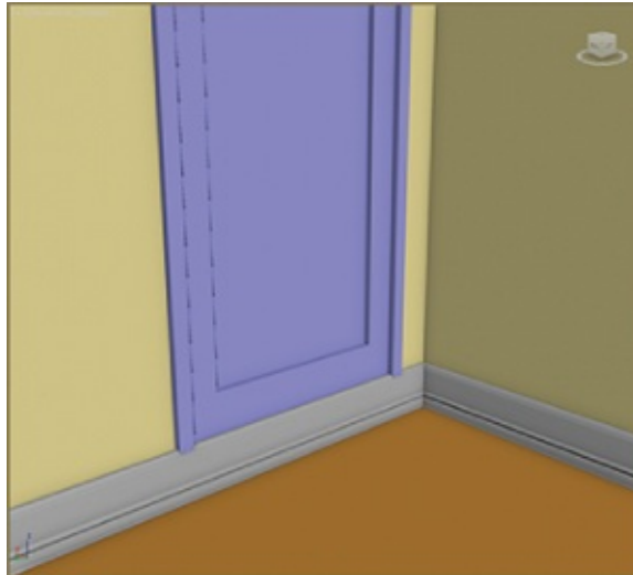
Figure 3.24 The baseboard molding is going through the door opening.
