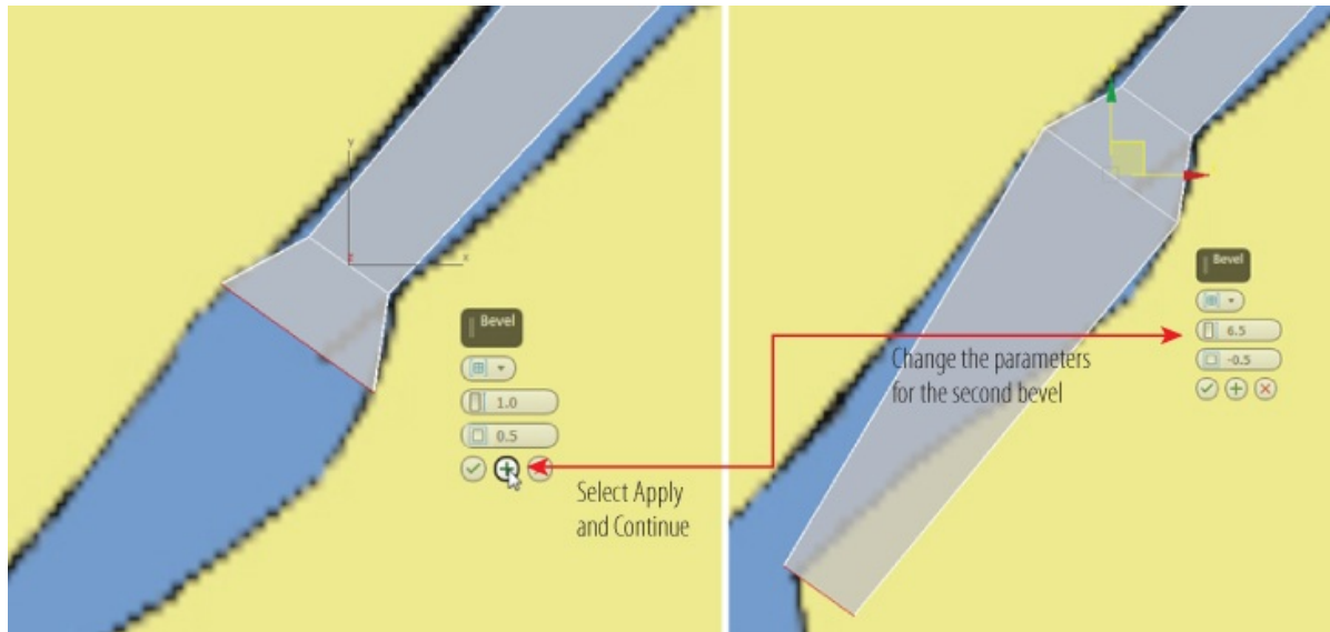
Figure 7.14 Bevel settings for completing the arm to the wrist
