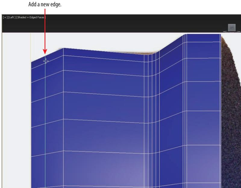
**FIGURE 2.17** Add an edge loop with SwiftLoop.
