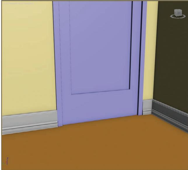
**FIGURE 3.26** The baseboard with proper gaps at doors
