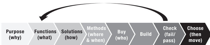
Figure 4.3 The W5H sequence: the stepwise process of evolving an idea into a product is recursively iterative
