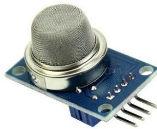
Gambar 2.3. Sensor MQ 2 (Hasibuan *et al.*, 2020)
