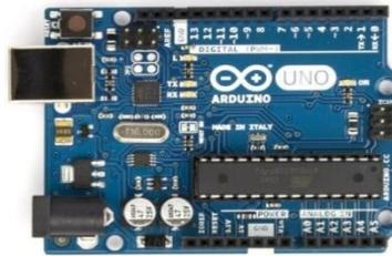
Gambar 2.1. Arduino Uno (Wasid, 2018)
