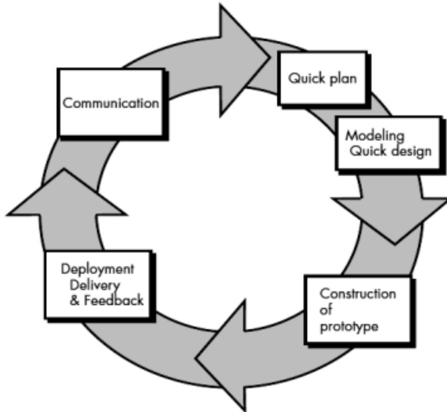
Gambar 2.1 Prototyping Model
