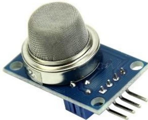
Gambar 2.1 Sensor MQ-135 (Sumber: Olimex, 2014)
