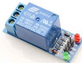
Gambar 2. 10 single channel relay ( https://www.elecrow.com )
