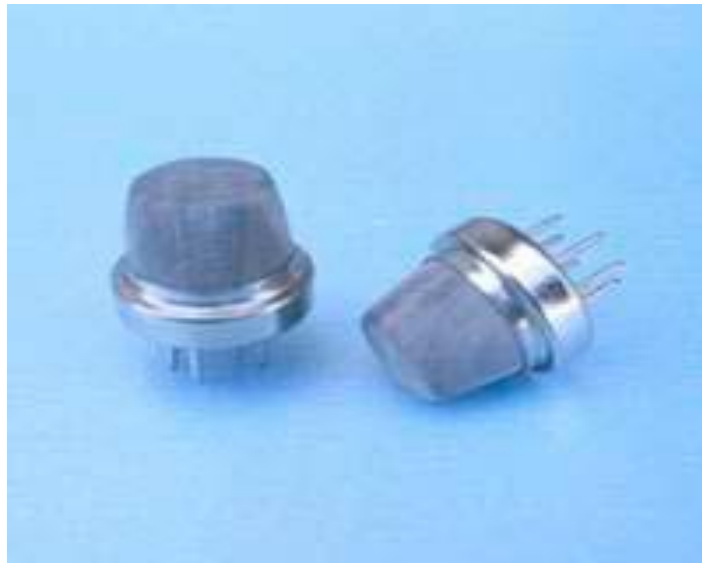
Gambar 2.1 Sensor MQ-135 (Sumber: Olimex, 2014)
