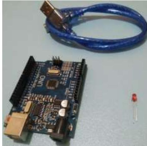
**Gambar 3.4** Arduino Uno Serta Lampu *LED (light-emitting diode)*
