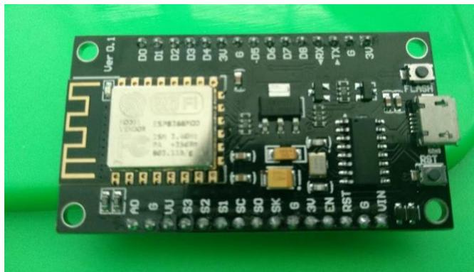
Gambar 2.4 NodeMCU ESP8266
