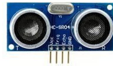
**Gambar 2.1 Sensor Ultraconic**
