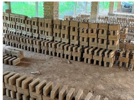
Gambar 2.4 Proses Penjemuran Bata
